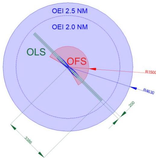
Figure 33 - Dimensions of the OEI and ICAO Annex 14 surfaces (2.5 NM and 2.0 NM)
