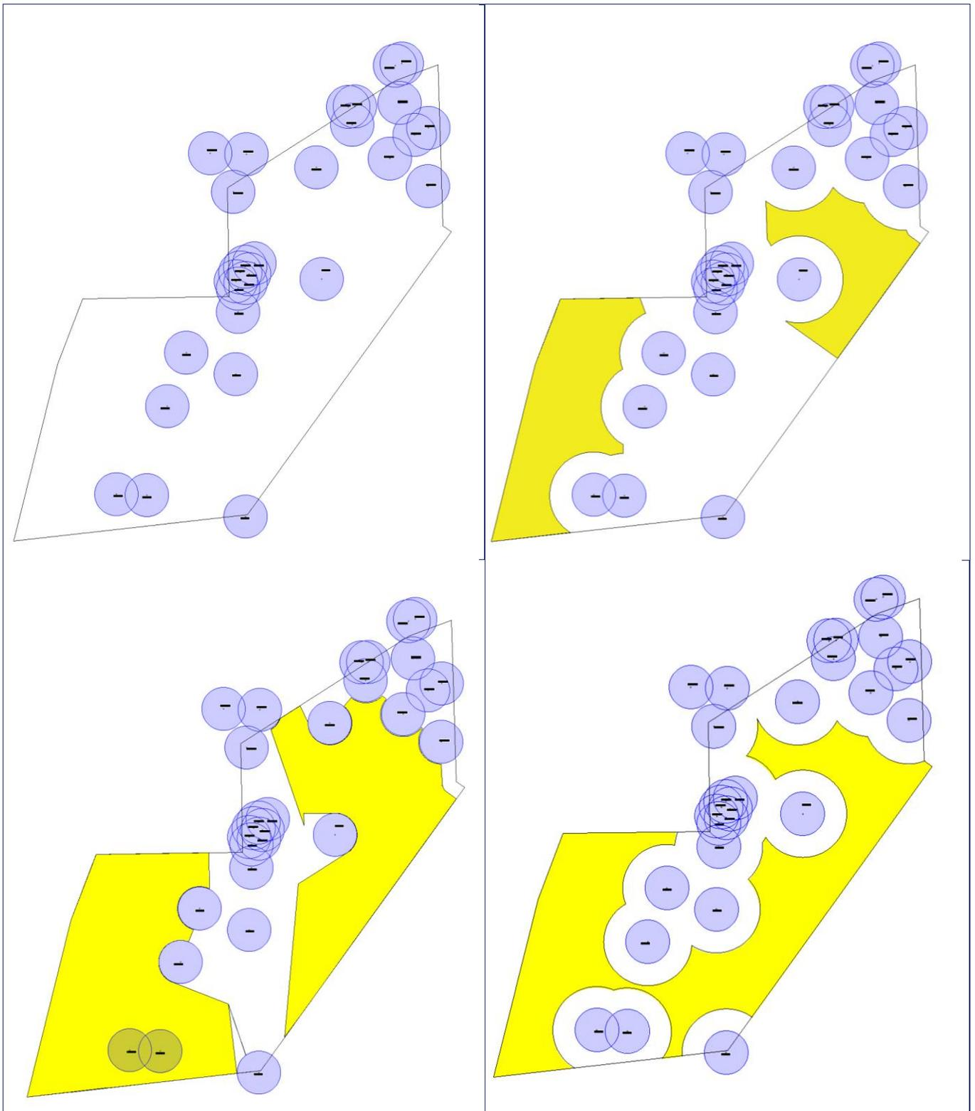
Figure 31 - Representation of the OEI area (based on a radius of 2.5 NM) required around each platform (top left), for combinativevariant 0 (top right), combinativevariant 27 (bottom left) and for the 5 NM scenario around the platforms (bottom right)
