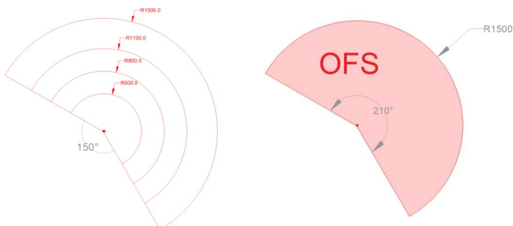
Figure 9 - 210-degree sector defined for different radius between 500 and 1500 m (for illustration purposes)
