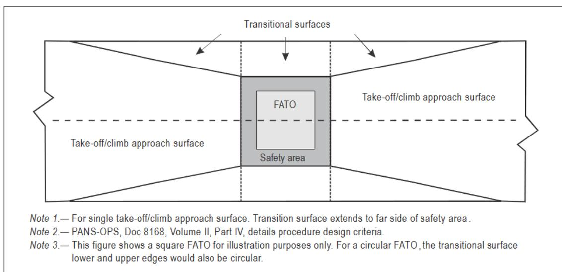
Figure 14 - Transitional surface for a FATO with a PinS approach procedure [Ref 1]
