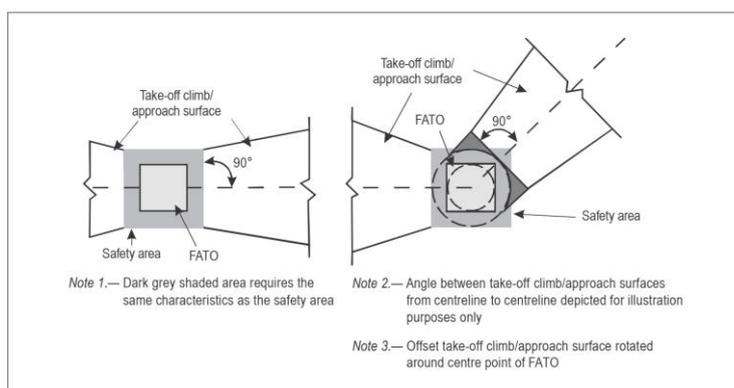
Figure 10 - Construction of take-off climb and approach surfaces [Ref 1]
