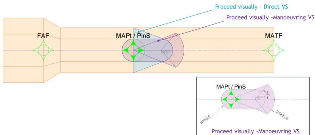
Figure 27 - Manoeuvring VS procedure option for the proceed visually approach
