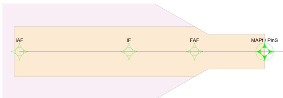
Figure 20 - Depiction of the area required for a PinS approach (IFR segment) based on RNP 0.3 (shown in orange) and RNP APCH (additional area shown in pink)
