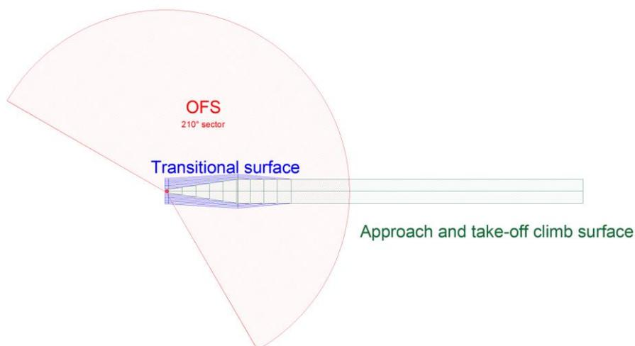
Figure 16 - Combination of all required ICAO Annex 14 surfaces for a generic case (single route)
