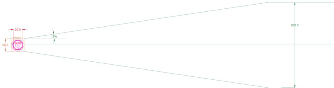
Figure 12 - Depiction of the initial segment of the approach and take-off climb surface
