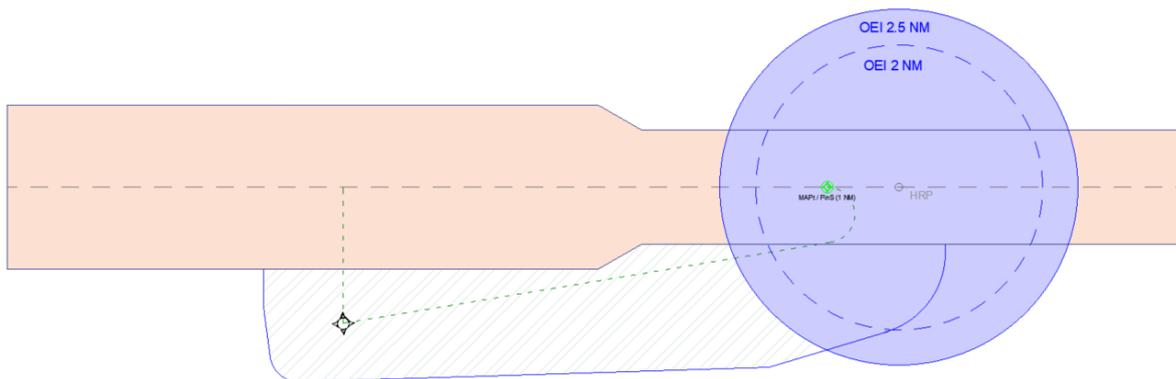
Figure 22 - Example of a turning missed approach and required additional area (depicted in green)
