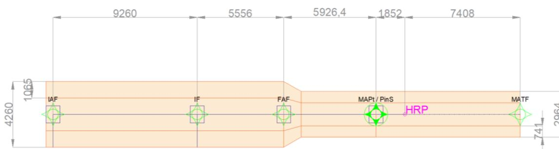
*Figure 21 - IFR segment of the PinS approach procedure (dimensions provided in meters)*
