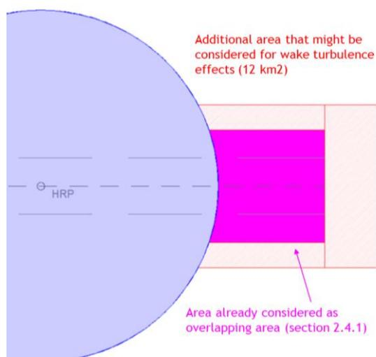
Figure 37 - Additional area to be considered for wake turbulence effects
