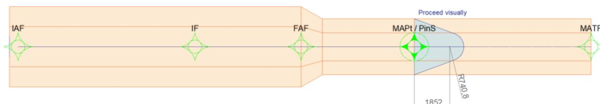
Figure 25 - Protection areas associated to the PinS approach (IFR segment and visual segment) for a proceed visually procedure
