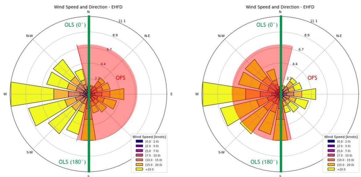
Figure 44 - Examples of two OFS and platform orientations for the provision of the same approach and take-off climb surfaces
