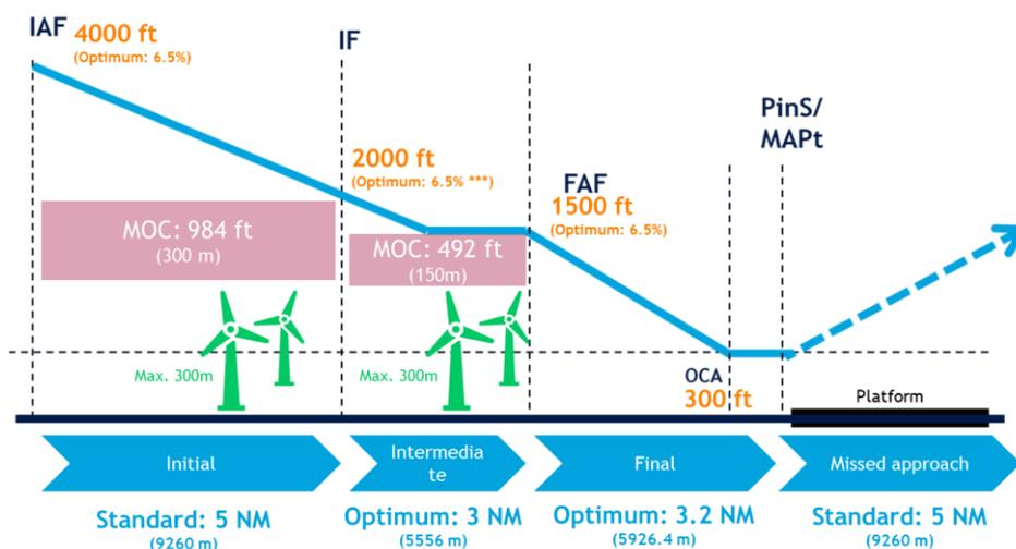
Figure 24 - Vertical representation of the standard IFR segment for a straight-in PinS approach (2000 ft)
