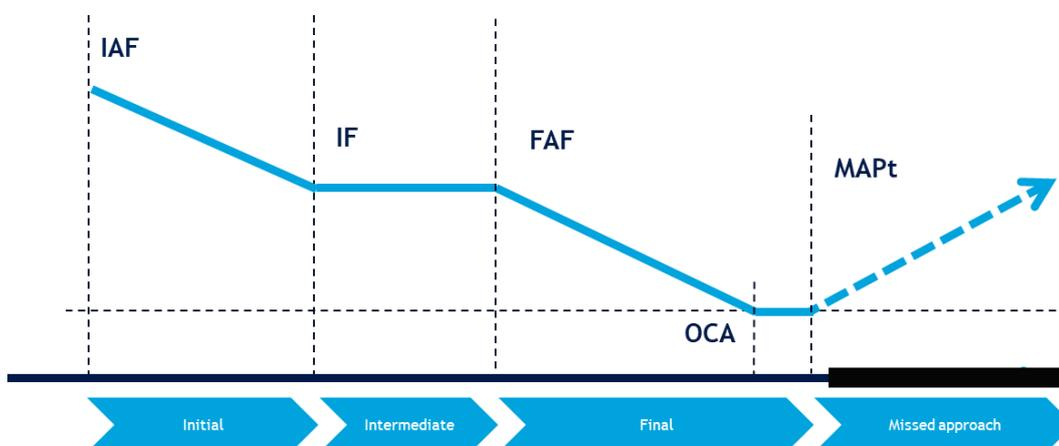
Figure 18 - Standard flight phases of an instrument approach procedure
