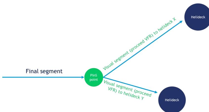
Figure 26 - Options in Proceed VFR to connect multiple platforms for a single IFR segment (from initial to final)
