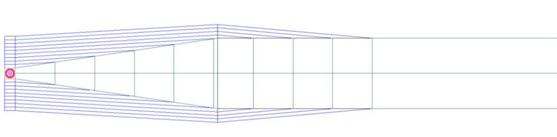
Figure 15 - Lateral definition of the transitional surface
