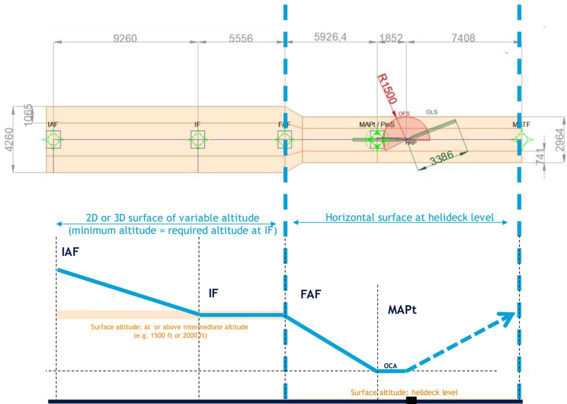
Figure 29 - Lateral and vertical representation of the required surfaces (ICAO Annex 14 and PANS-OPS)
