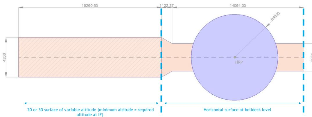
Figure 35 - Total area required based on the combination of PinS and OEI procedures
