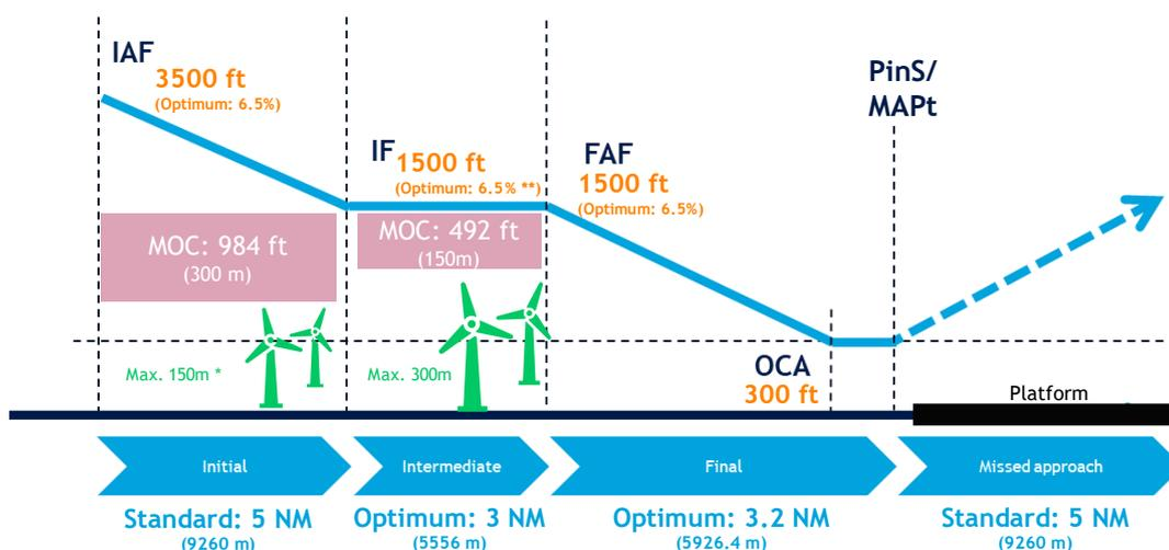
Figure 23 - Vertical representation of the standard IFR segment for a straight-in PinS approach (1500 ft)
