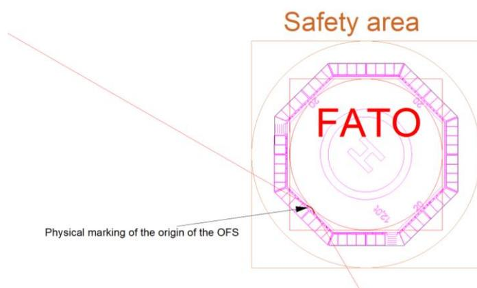
Figure 8 - Physical marking of the origin of the OFS
