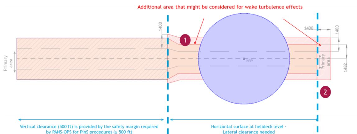
Figure 36 - Effect of wake turbulence and additional margins needed
