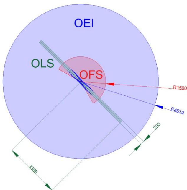
Figure 32 - Dimensions of the OEI and ICAO Annex 14 surfaces (2.5 NM)
