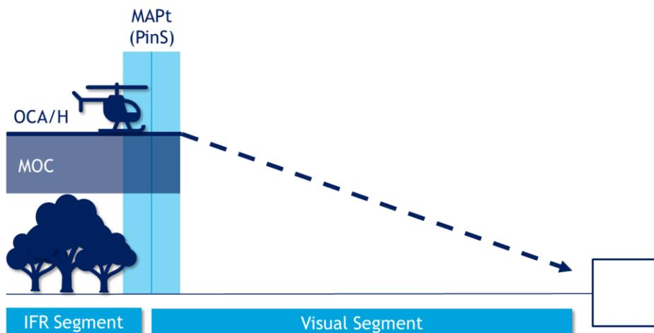
Figure 19 - Generic PinS approach procedure
