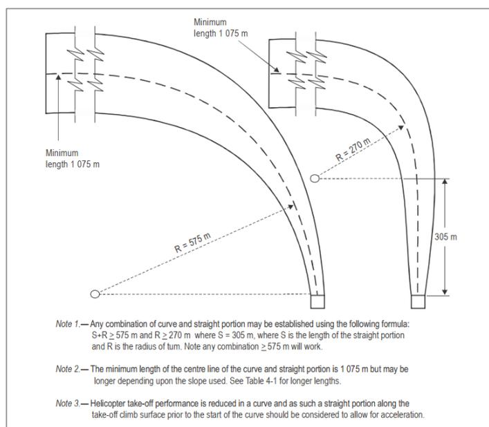
Figure 11 - Requirements for turn dimensions on approach and take-off routes [Ref 1]
