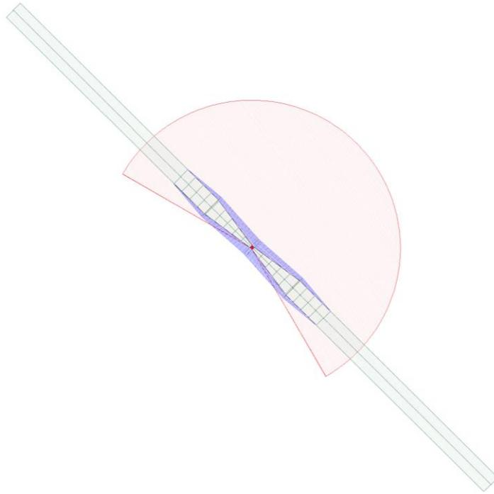
Figure 17 - Combination of all required ICAO Annex 14 surfaces for a generic case (two routes)
