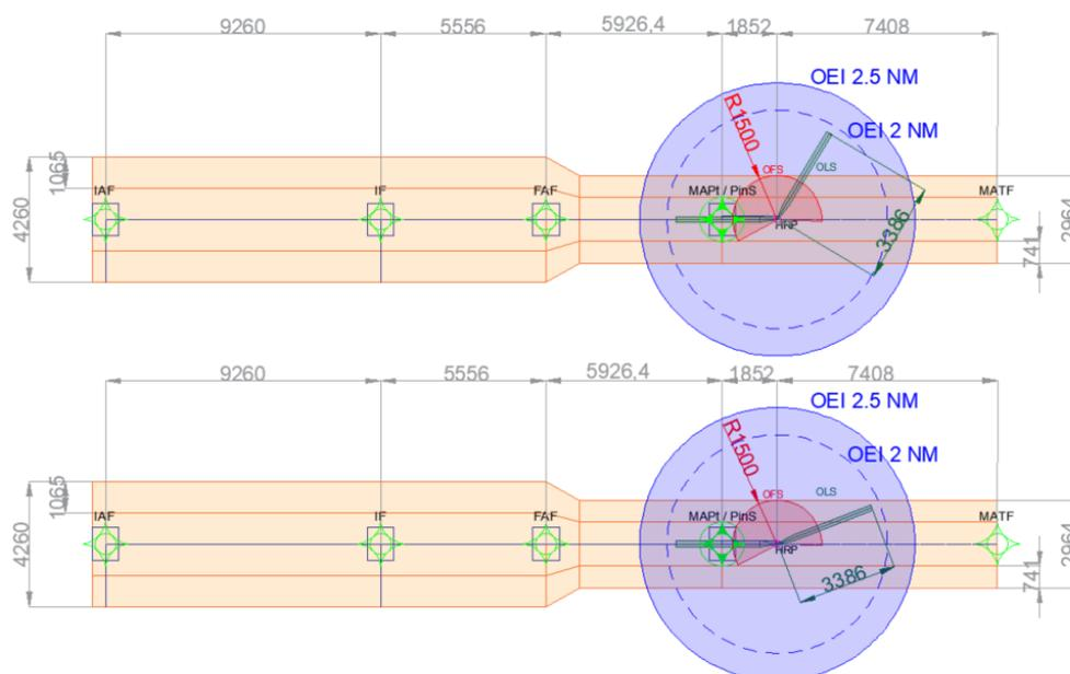
Figure 34 - Depiction of a standard PinS approach procedure with some examples of OFS and OLS and the two scenarios considered for OEI (2.5 and 2 NM)
