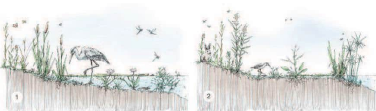
Figuur 6-13 - 1) plasberm, 2) drasberm (Stowa, 2009)
