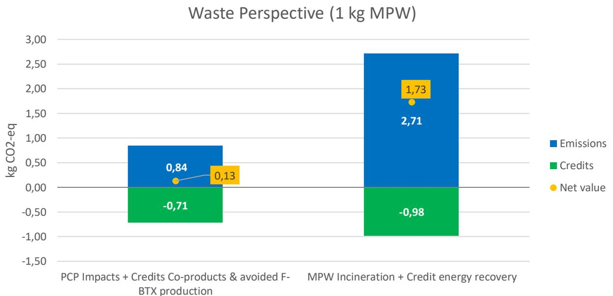
Figure 3 Results from the LCA in which the PCP process on the left is compared with the Business-as-usual on the right. For this perspective the MPW is processed in a waste-to-energy plant and is referred here as incineration of the MPW. In blue the emissions of both processes are given. In green the credits (avoided production of substitute processes) are given. When the emissions and credits are combined the resulting impact is shown as a yellow dot in the bar.
