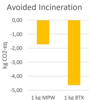
Figure 15 Environmental credits for avoided incineration for the global warming potential in kg of CO<sub>2</sub>-equivalents. On the left are the credits shown for the waste perspective (1 kg MPW) and on the right for the product perspective (1 kg BTX).
