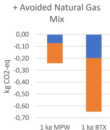
Figure 13 Global warming potential credits for avoided natural gas mix, added to the previous process in kg of CO<sub>2</sub>-equivalents. On the left are the credits shown for the waste perspective (1 kg MPW) and on the right for the product perspective (1 kg BTX).
