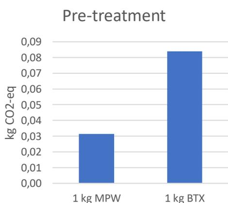
Figure 7 Global warming impact for the pre-treatment step of the process in kg CO<sub>2</sub>-equivalents. The left figure represents the waste perspective (1 kg MPW) and the right figure represents the product perspective (1 kg R-BTX). For 1 kg BTX, ~2.68 kg MPW is needed.
