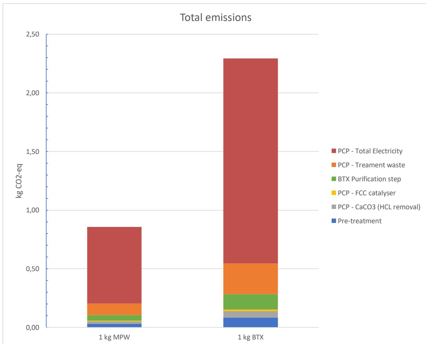
Figure 12 Total impacts of both perspectives in kg of CO<sub>2</sub>-equivalents. The left bar represents the waste perspective (1 kg MPW) and the right bar represents the product perspective (1 kg BTX). For 1 kg R-BTX, ~2.68 kg MPW is needed.
