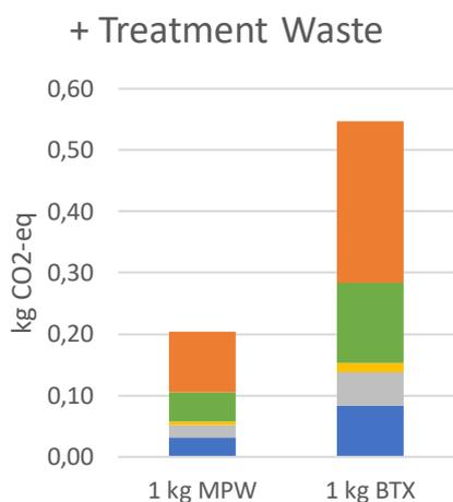
Figure 10 Total impact of the previous processes and added treatment of waste fractions in kg of CO<sub>2</sub>-equivalents. The left bar represents the waste perspective (1 kg MPW) and the right bar represents the product perspective (1 kg BTX). For 1 kg R-BTX, ~2.68 kg MPW is needed.
