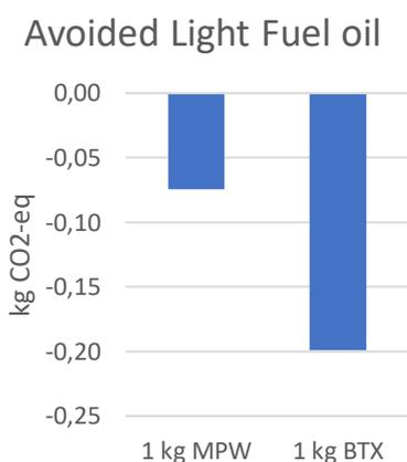
Figure 14 Global warming potential credits for avoided light fuel production in kg of CO<sub>2</sub>-equivalents. On the left are the credits shown for the waste perspective (1 kg MPW) and on the right for the product perspective (1 kg BTX).
