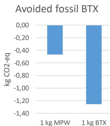
Figure 16 Environmental credits for avoided fossil BTX production for the global warming potential in kg of CO<sub>2</sub>-equivalents. On the left are the credits shown for the waste perspective (1 kg MPW) and on the right for the product perspective (1 kg BTX).
