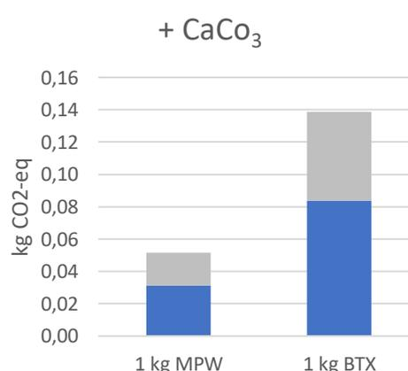
Figure 6 Total impact of the pre-treatment and added production of CaCO<sub>3</sub> in kg CO<sub>2</sub>-eq. The left figure represents the waste perspective (1 kg MPW) and the right figure represents the product perspective (1 kg R-BTX). For 1 kg R-BTX, ~2.68 kg MPW is needed.
