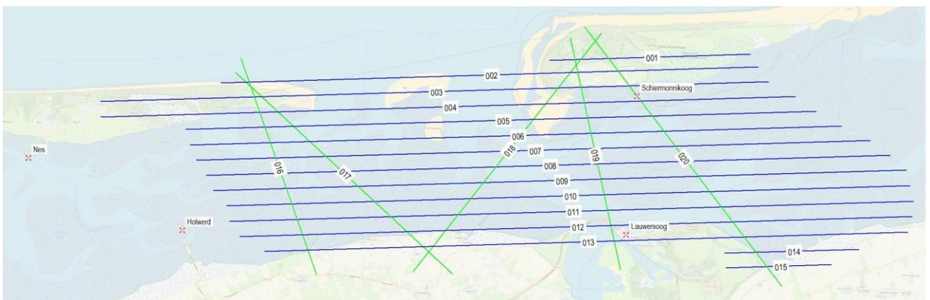
Figure 4: Flightplan and waterlevel stations
