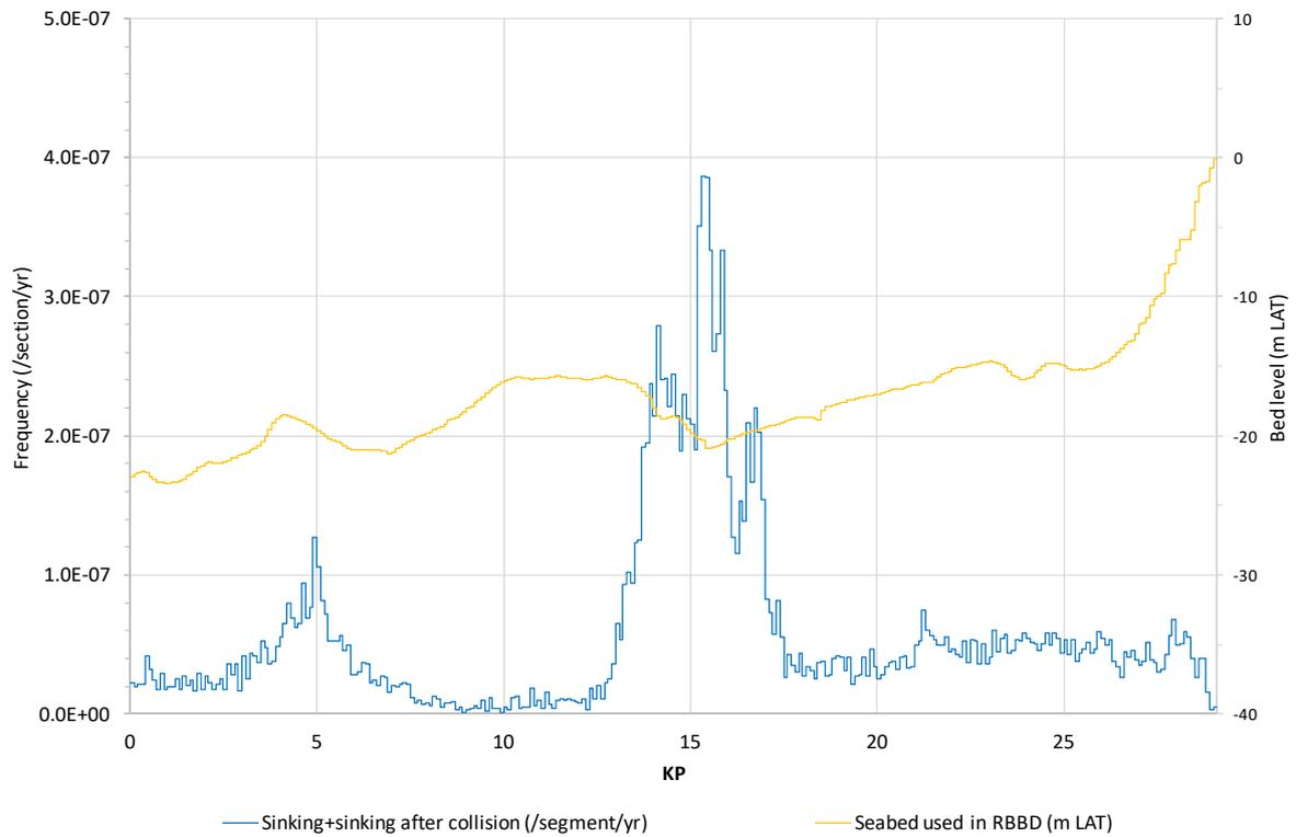
**Figure A2.8** Frequency that critical ship sinking occurs on **Hollandse Kust (noord) route alternative 2.**
