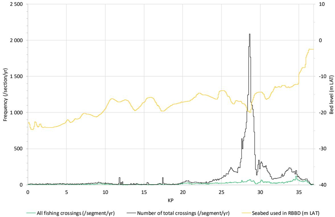
**Figure A2.5** Frequency of all the ships (black line) and fishing ships (green line) that cross **Hollandse Kust (noord) route alternative 6** (/section/yr) as function of the cable route (KP). Note: The scale of the y-axis is a factor 10 larger compared to routes 1-5.
