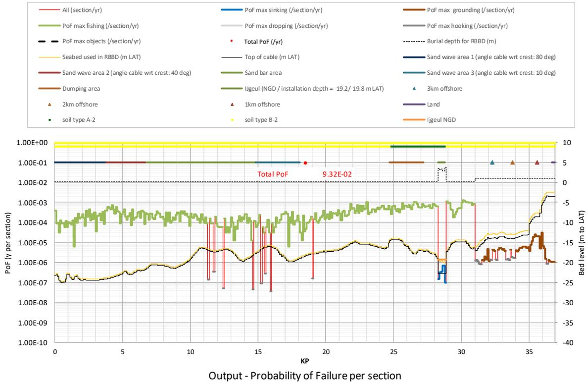
**Figure A2.53** Probability of Failure (PoF) for *Hollandse Kust (noord)* route alternative 6: Minimum scenario = burial scenario 2 + pre-sweeping, burial depth is 1 m (nearshore, < 3km from shore), 0.3 m (offshore, > 3km), burial in IJ-geul 3m below -19.8 m LAT (= NGD-0.5m)
