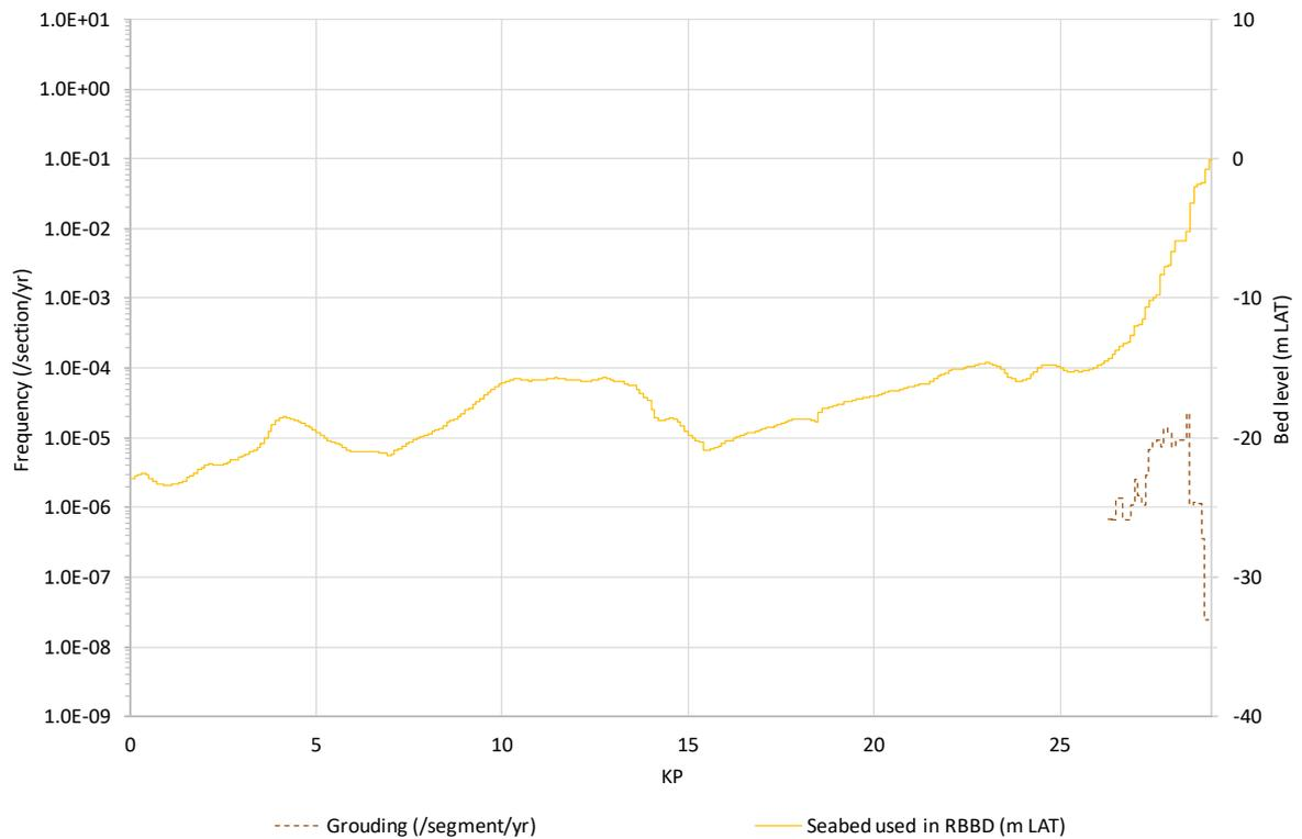
**Figure A2.14** Frequency that critical ship grounding occurs on *Hollandse Kust (noord)* route alternative 2.
