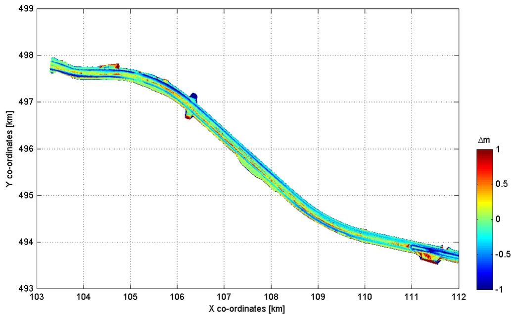
Figure 4.8: Bed level difference in Noordzeekanaal between 2009 and 2017.
