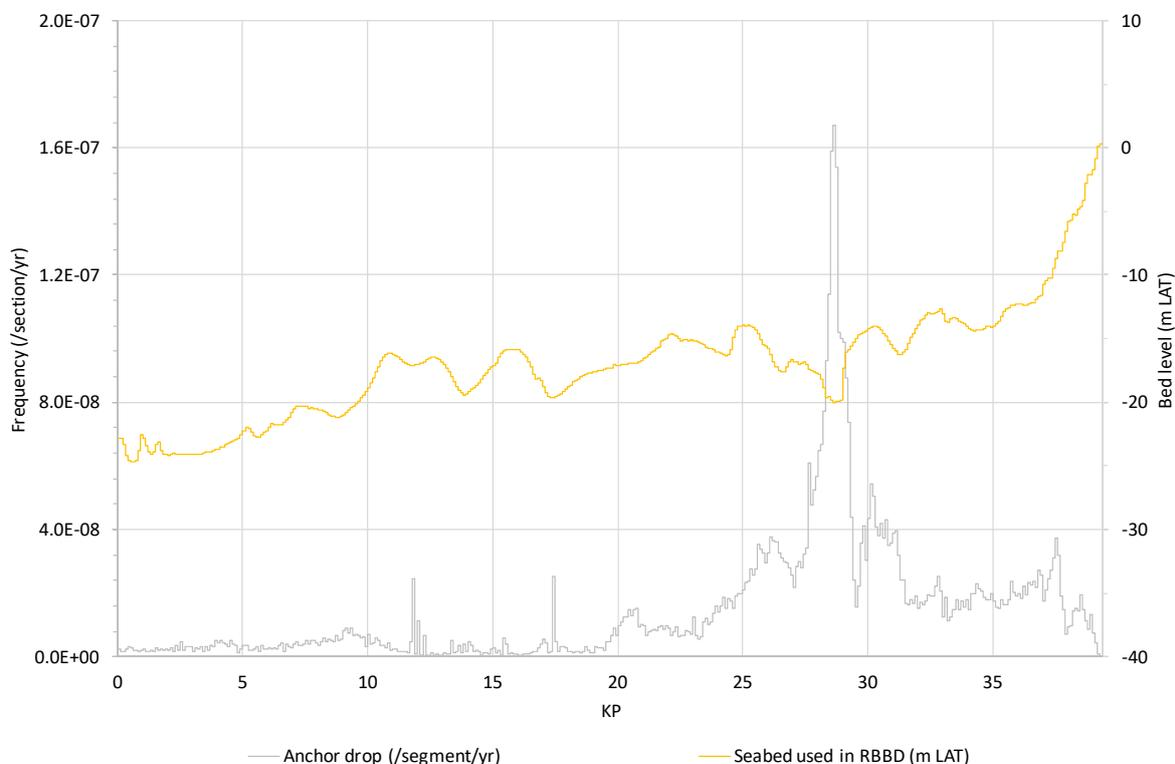
**Figure A2.24** Frequency that critical anchor dropping occurs on **Hollandse Kust (noord) route alternative 7**. Note: The scale of the y-axis is a factor 2 larger compared to routes 1-5.
