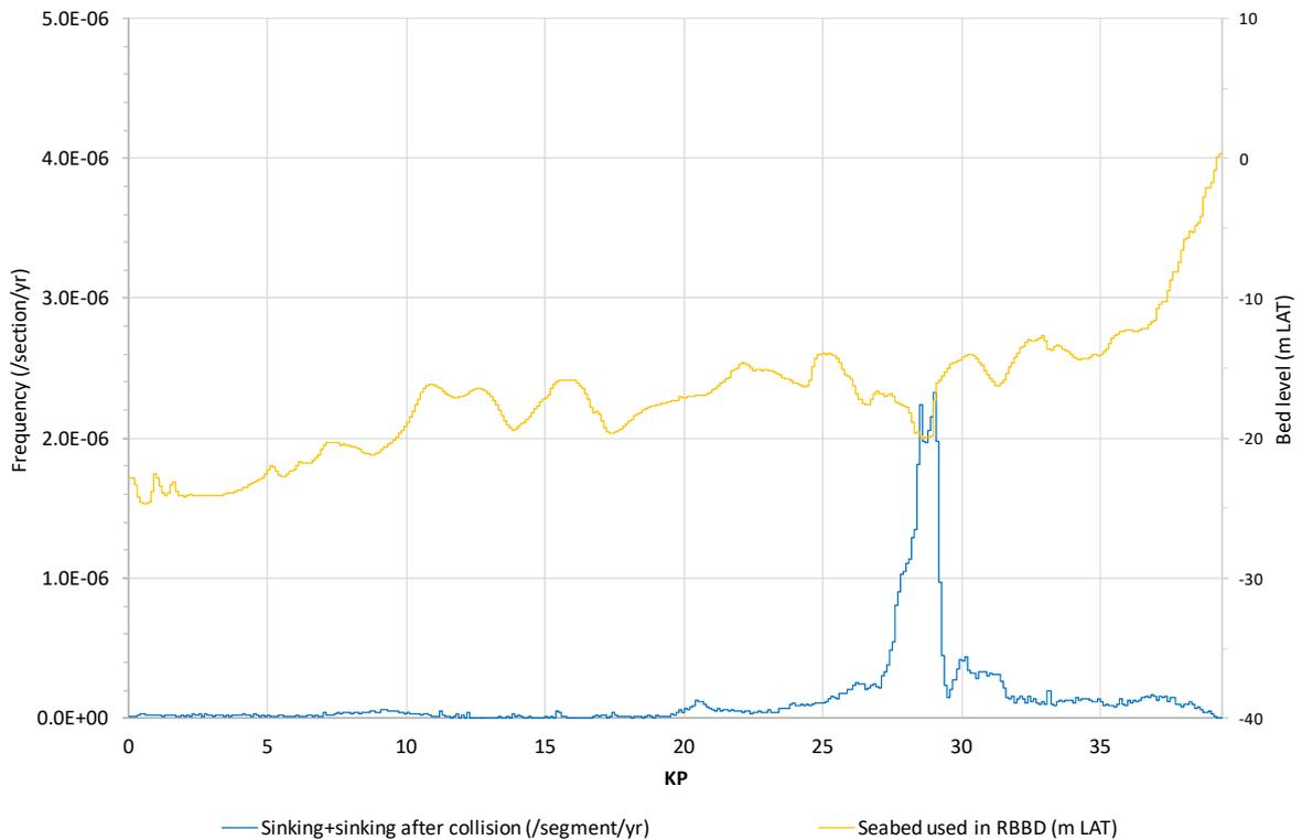
**Figure A2.12** Frequency that critical ship sinking occurs on **Hollandse Kust (noord) route alternative 7**. Note: The scale of the y-axis is a factor 10 larger compared to routes 1-5.
