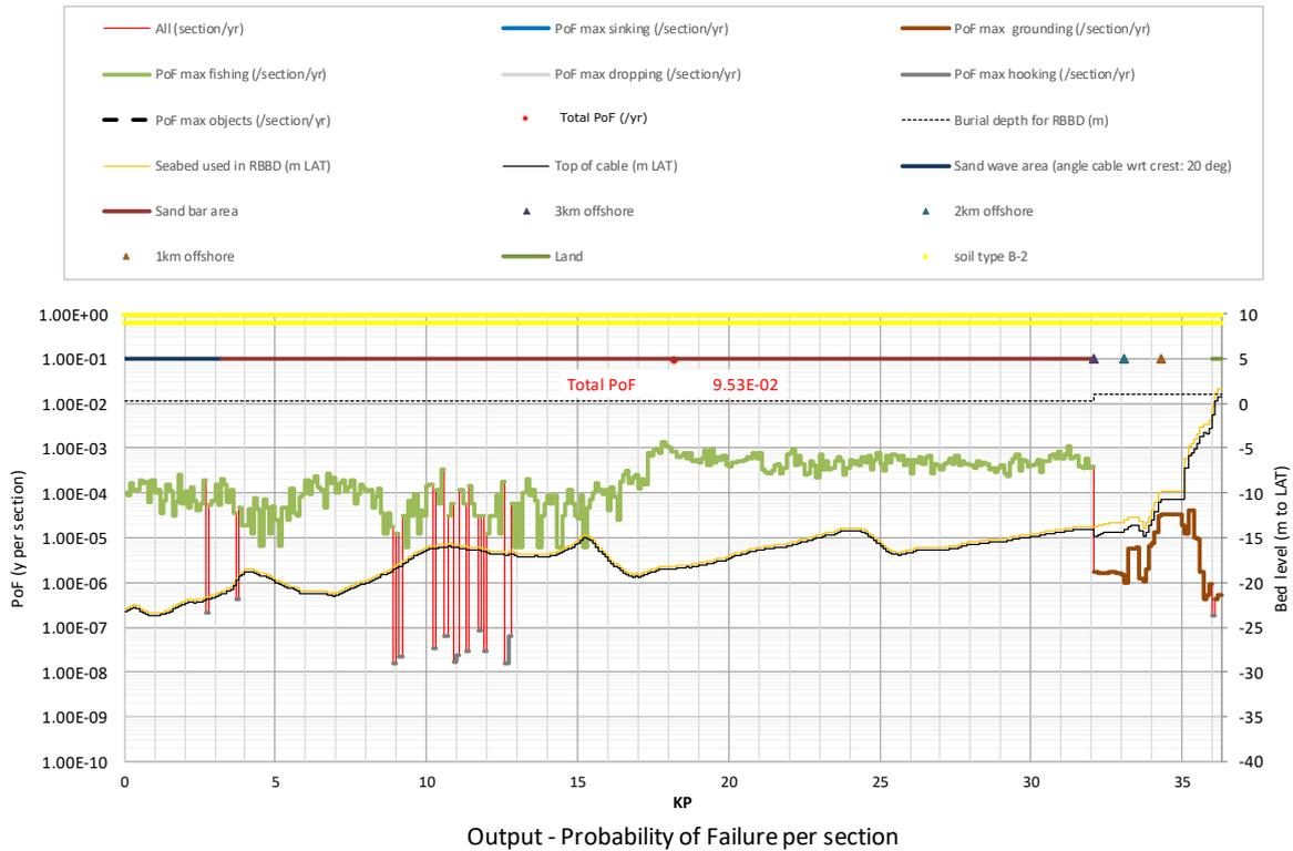
**Figure 7.3** Probability of Failure (PoF) for Hollandse Kust (noord) route alternative 4: Minimum scenario: Burial depth is 1 m (KP>32.1), 0.3 m (KP<32.1).
