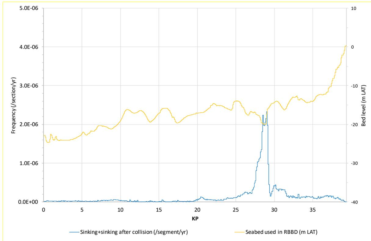
**Figure 5.4** Frequency that critical ship sinking occurs on the Hollandse Kust (noord) route alternative 7.
