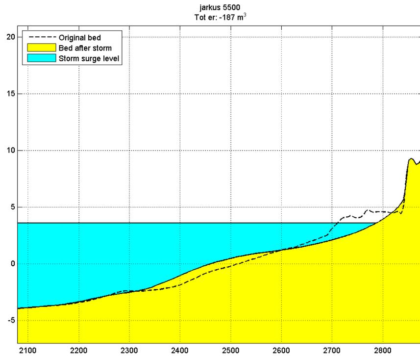
Figure 3.20: Model results of the impact of a 1/100 years storm condition on the most recent recorded coastal profile at landfall location 4+5.
