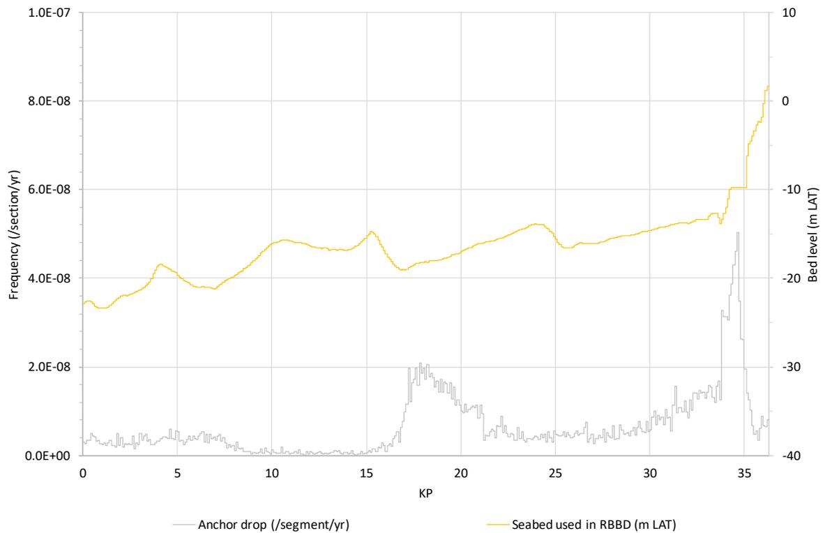
**Figure A2.22** Frequency that critical anchor dropping occurs on *Hollandse Kust (noord)* route alternative 4 and 5.
