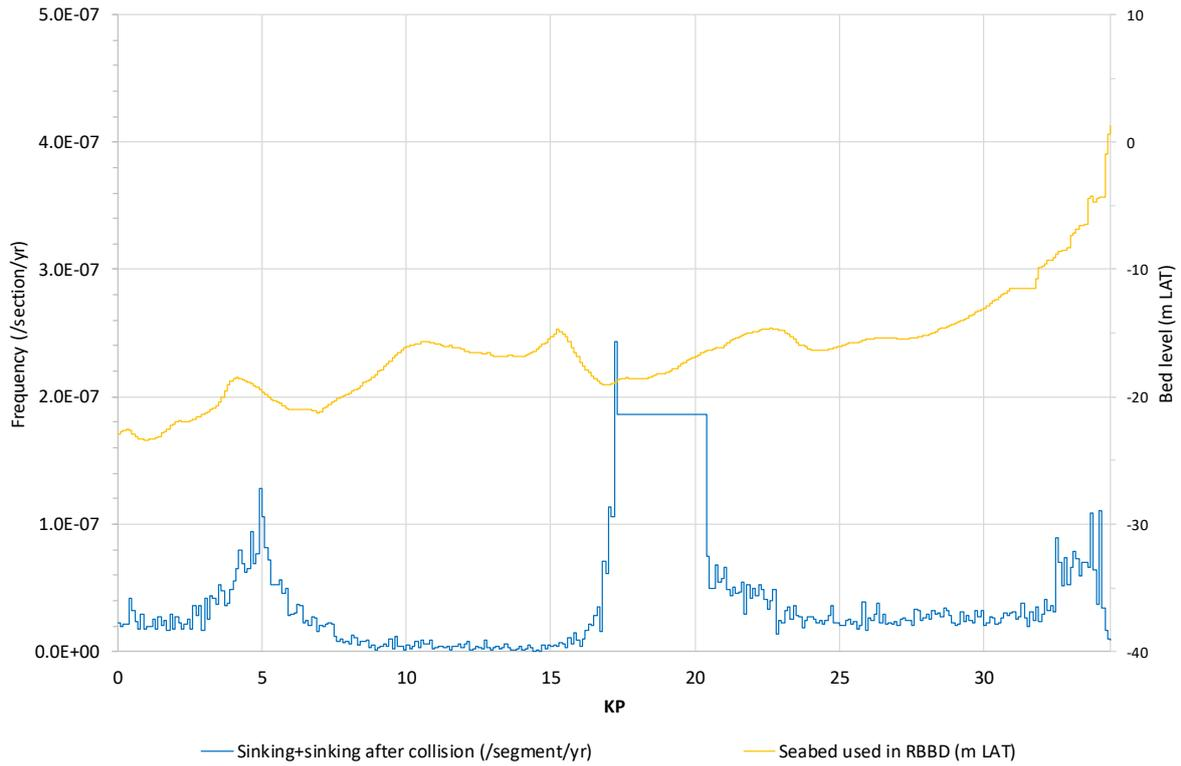
**Figure A2.9** Frequency that critical ship sinking occurs on *Hollandse Kust (noord) route alternative 3*.
