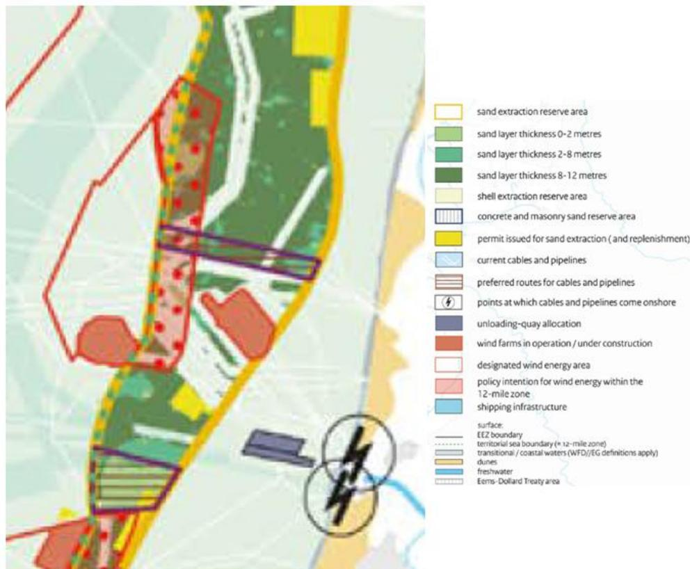
Figure 2.13 Sand extraction strategy map zoomed in on area around wind farm HKN with permitted sand extraction areas indicated in yellow and sand disposal areas indicated in dark blue. Source: [https://www.noordzeeloket.nl/en/Images/Sand%20extraction%20strategy\\_4923.pdf](https://www.noordzeeloket.nl/en/Images/Sand%20extraction%20strategy_4923.pdf) (visited 24 August 2017)
