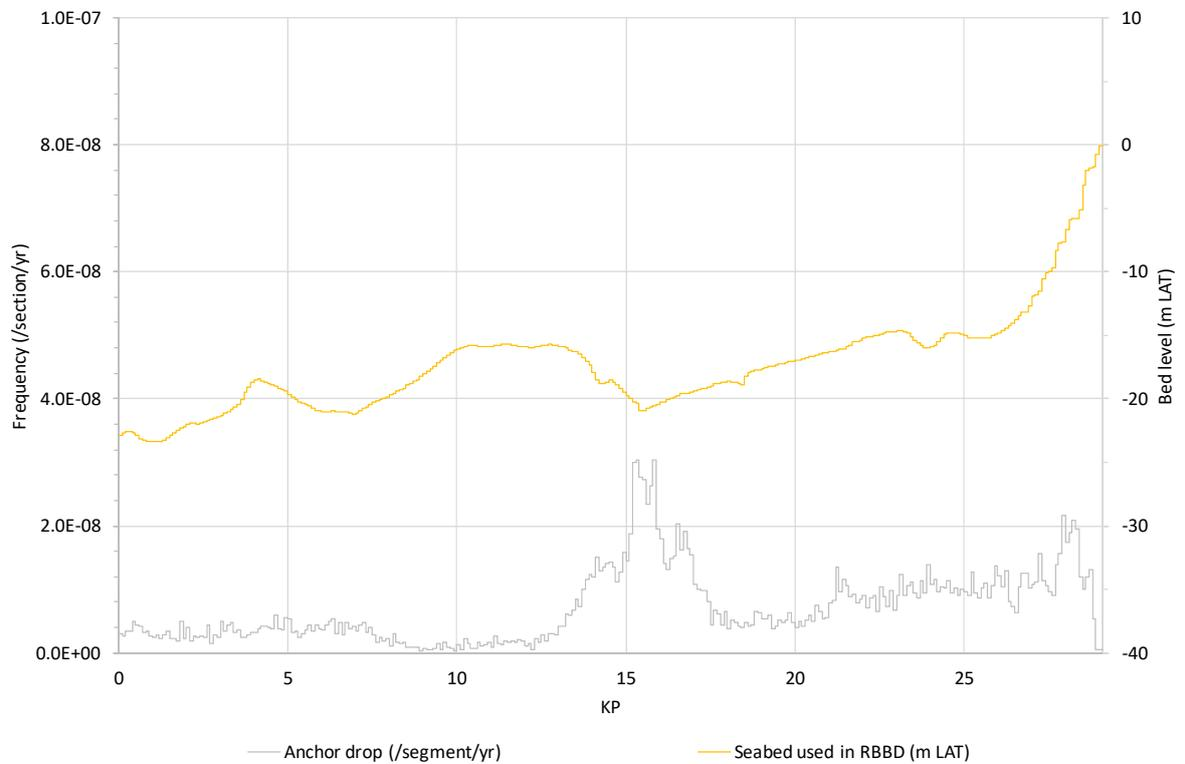
**Figure A2.20** Frequency that critical anchor dropping occurs on *Hollandse Kust (noord)* route alternative 2.
