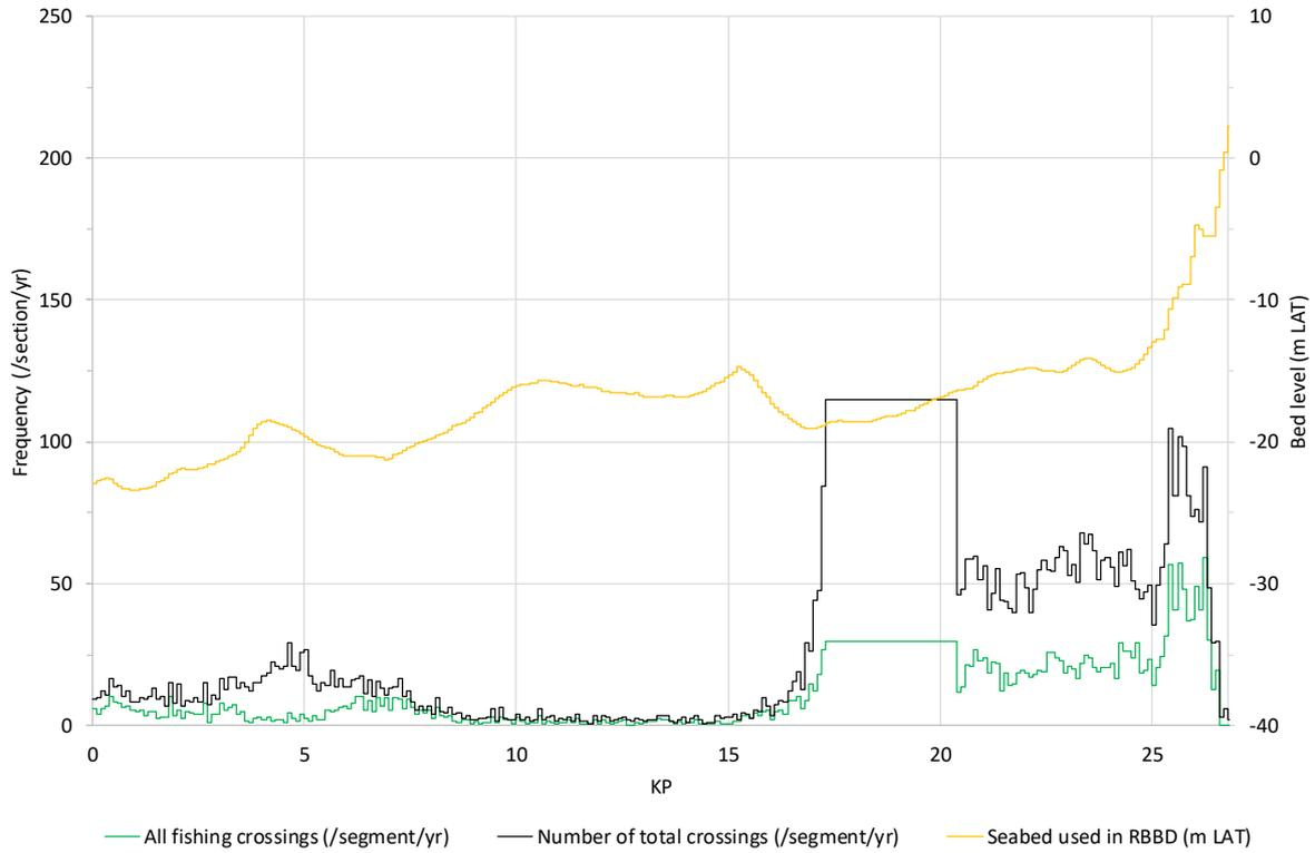
**Figure A2.1** Frequency of all the ships (black line) and fishing ships (green line) that cross **Hollandse Kust (noord) route alternative 1** (/segment/yr) as function of the cable route (KP). The numbers are based on two year of AIS data (from 1 August 2013 to 1 August 2015) for each segment of ~100 m.
