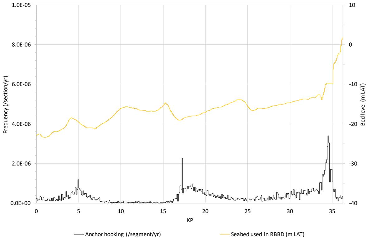
**Figure 5.12** Frequency that critical anchor hooking occurs on Hollandse Kust (noord) route alternative 4.
