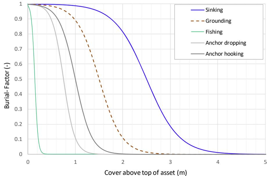
**Figure 6.1** *Burial-Factors for sinking, grounding, anchor hooking, anchor dropping and bottom trawling for the B-2 Medium Loose Sand, as function of cover above the cable.*
