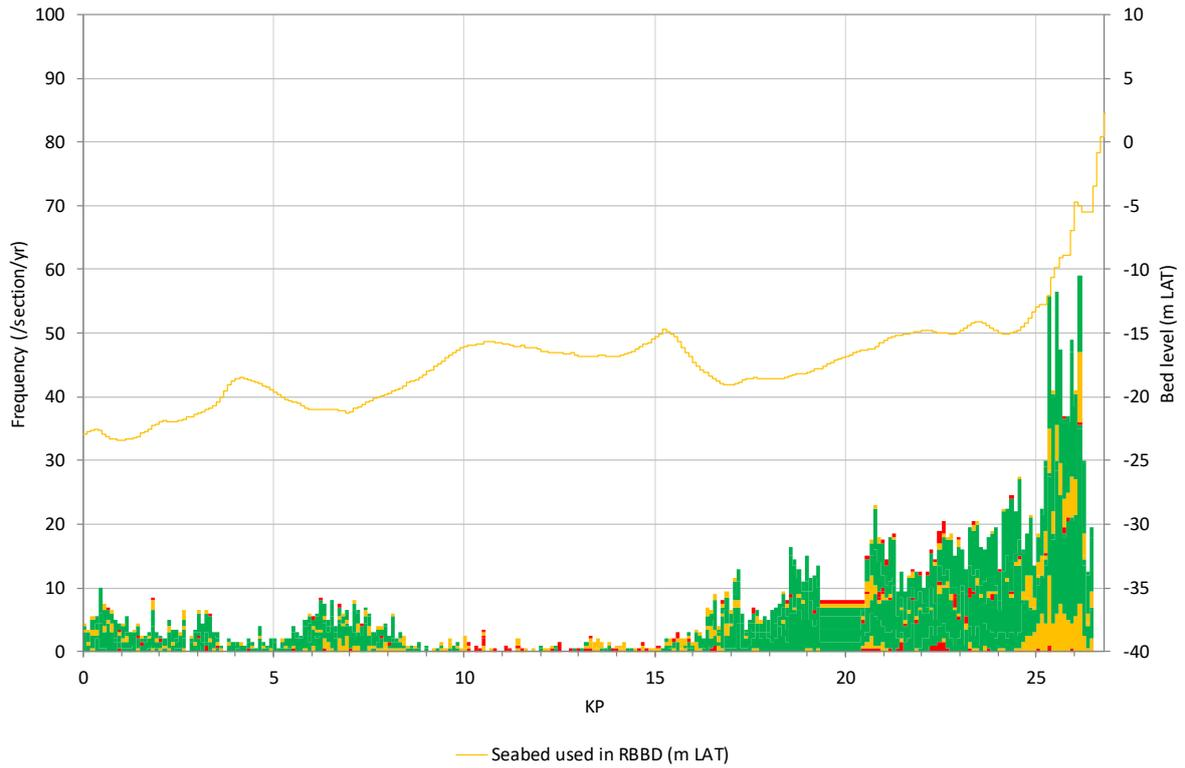
**Figure A2.31** Frequency that fishing activities interacting with *Hollandse Kust (noord)* route alternative 1.
