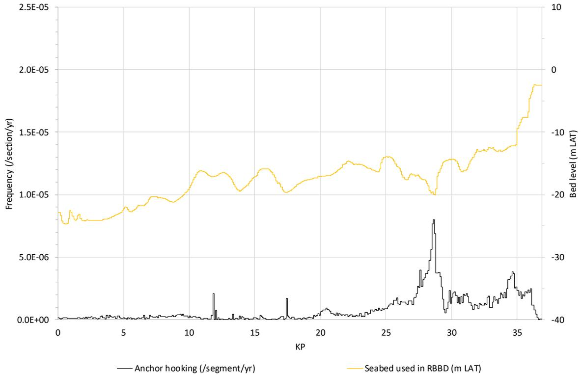
**Figure A2.29** Frequency that critical anchor hooking occurs on **Hollandse Kust (noord) route alternative 6**. Note: The scale of the y-axis is a factor 2 larger compared to routes 1-5.
