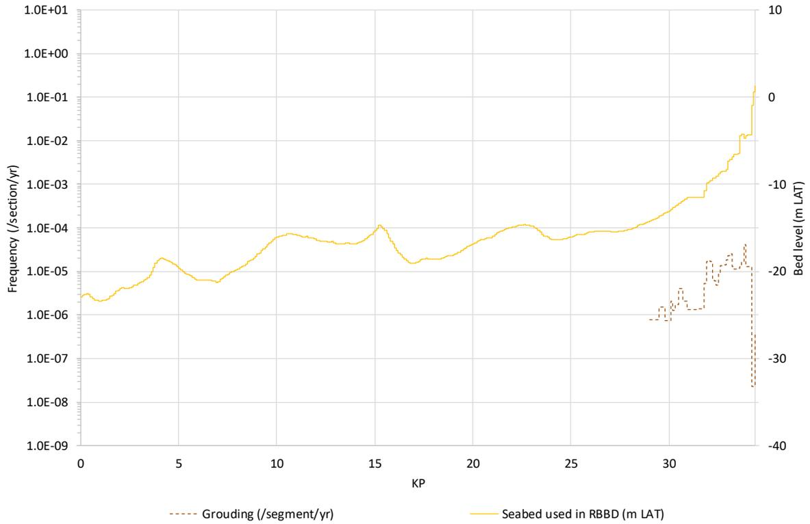
**Figure A2.15** Frequency that critical ship grounding occurs on *Hollandse Kust (noord)* route alternative 3.
