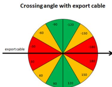
**Figure 5.17** Crossing angles of fishing vessels with respect to the export cable.
