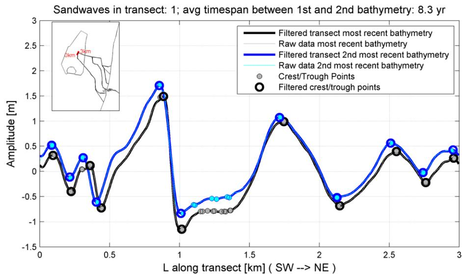
Figure 2.10 Fourier filtered sand waves along transect 1
