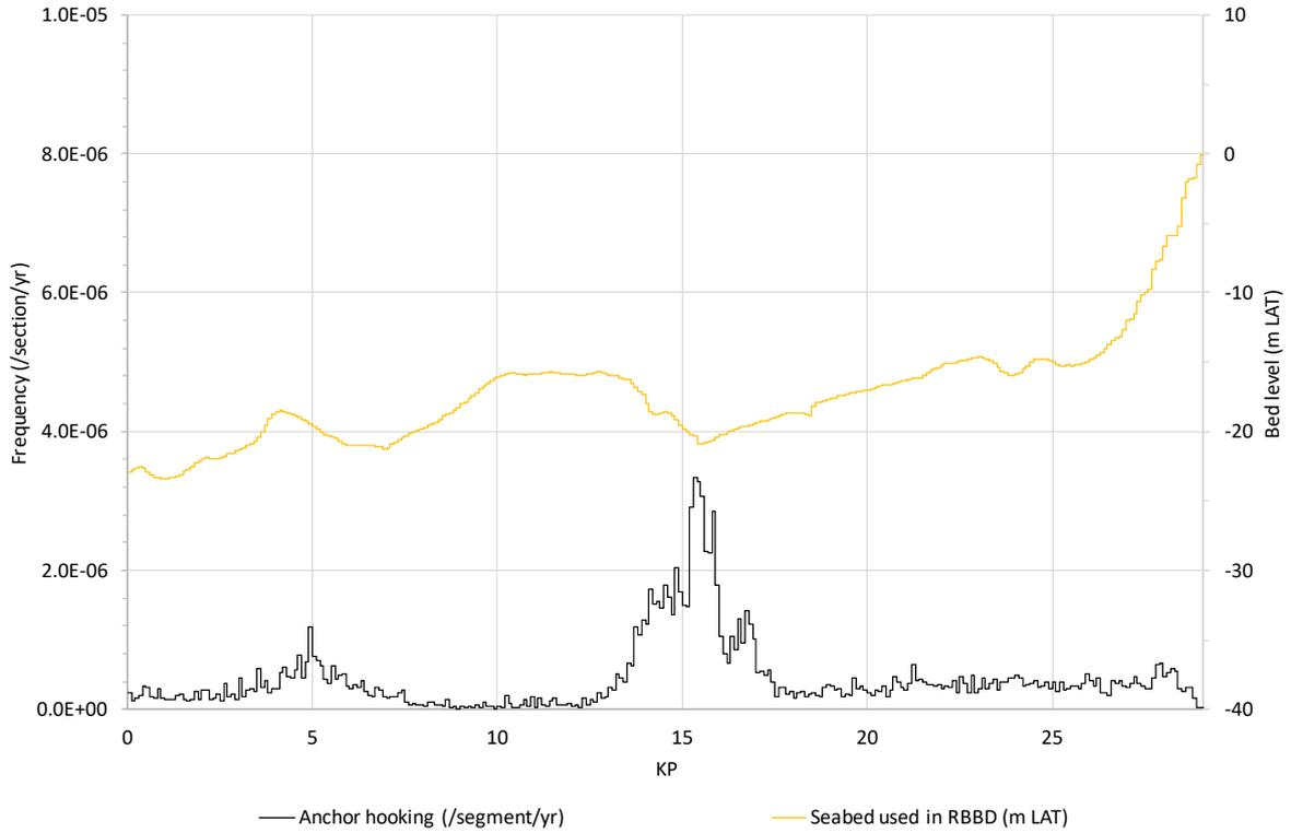
**Figure 5.11** Frequency that critical anchor hooking occurs on Hollandse Kust (noord) route alternative 2.
