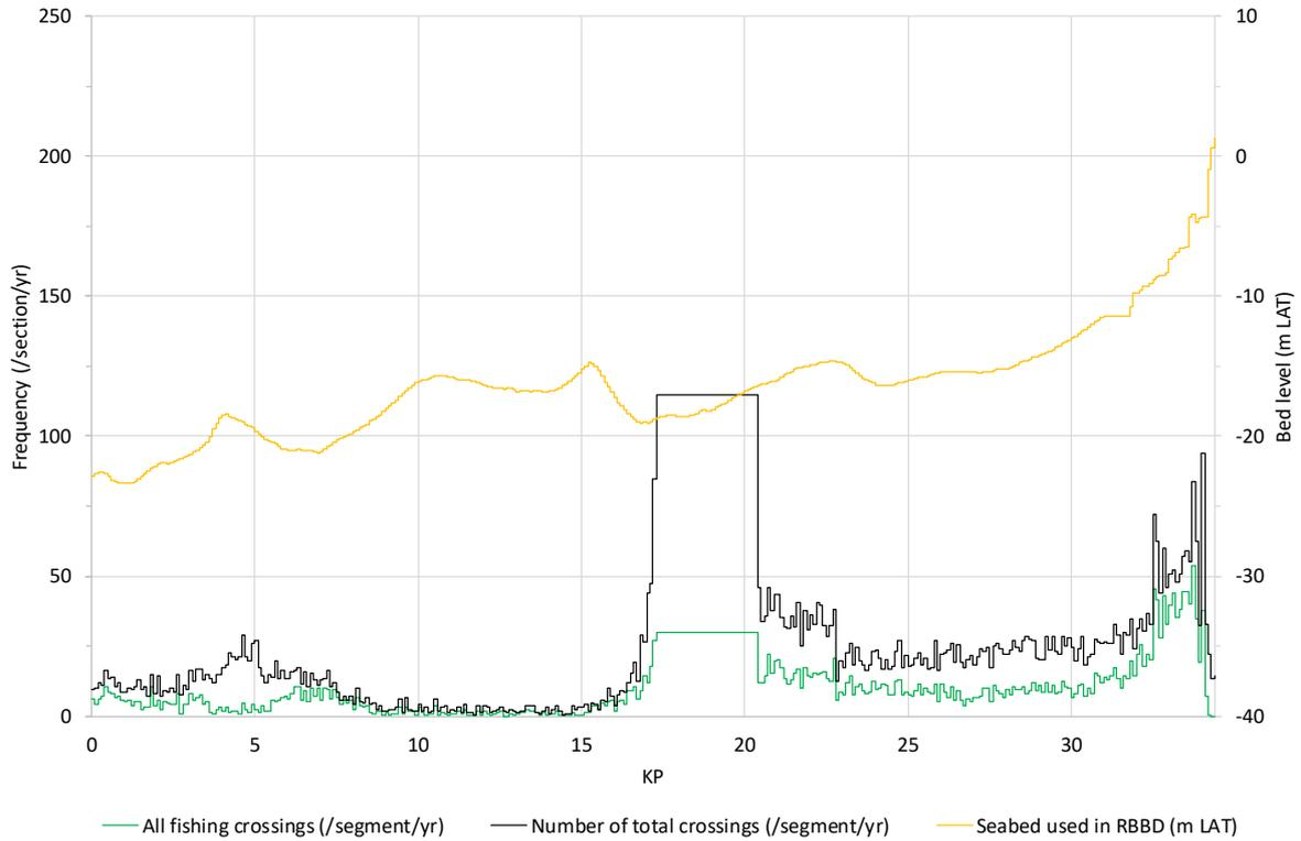
**Figure A2.3** Frequency of all the ships (black line) and fishing ships (green line) that cross **Hollandse Kust (noord) route alternative 3** (/section/yr) as function of the cable route (KP).
