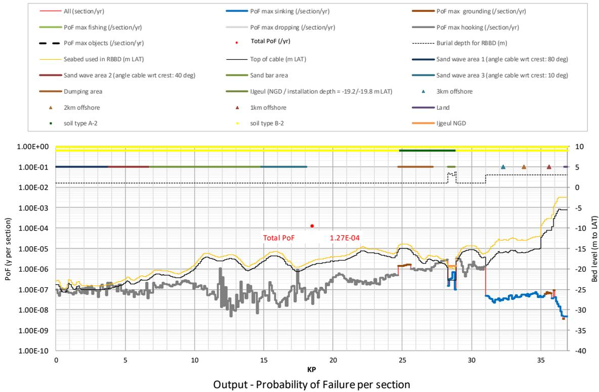
**Figure A2.41** Probability of Failure (PoF) for *Hollandse Kust (noord)* route alternative 6: Installation scenario = Initial permitting requirements + pre-sweeping, burial depth is 3 m (nearshore, < 3km from shore), 1 m (offshore, > 3km), burial in IJ-geul is 3m below -19.8 m LAT (= NGD-0.5m)
