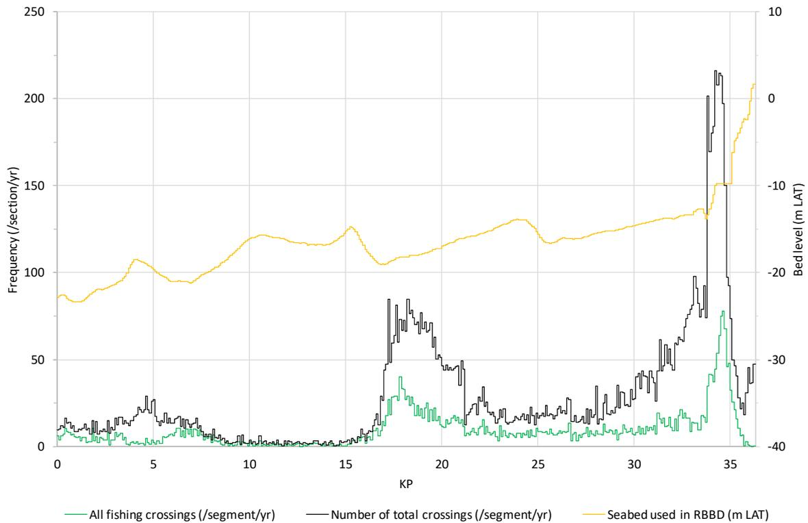
**Figure A2.4** Frequency of all the ships (black line) and fishing ships (green line) that cross **Hollandse Kust (noord) route alternative 4 en 5** (/section/yr) as function of the cable route (KP).
