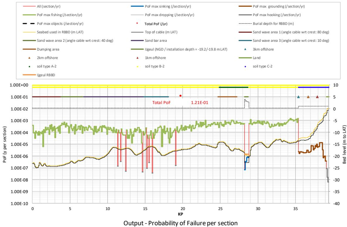
**Figure A2.54** Probability of Failure (PoF) for *Hollandse Kust (noord)* route alternative 7: Minimum scenario = burial scenario 2 + pre-sweeping, burial depth is 1 m (nearshore, < 3km from shore), 0.3 m (offshore, > 3km), burial in IJ-geul 3m below -19.8 m LAT (= NGD-0.5m)
