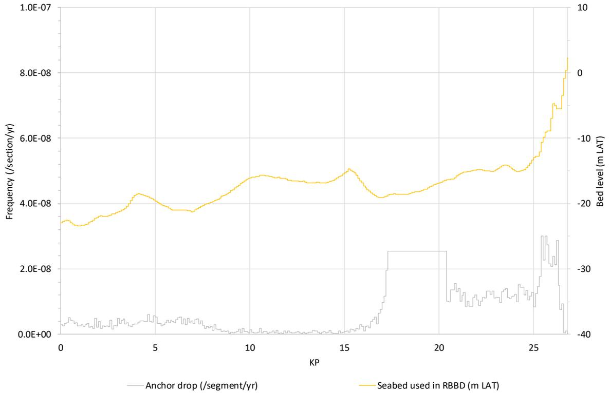
**Figure A2.19** Frequency that critical anchor dropping occurs on *Hollandse Kust (noord)* route alternative 1.
