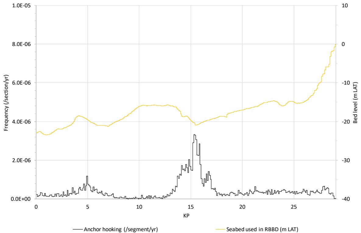
**Figure A2.26** Frequency that critical anchor hooking occurs on *Hollandse Kust (noord)* route alternative 2.
