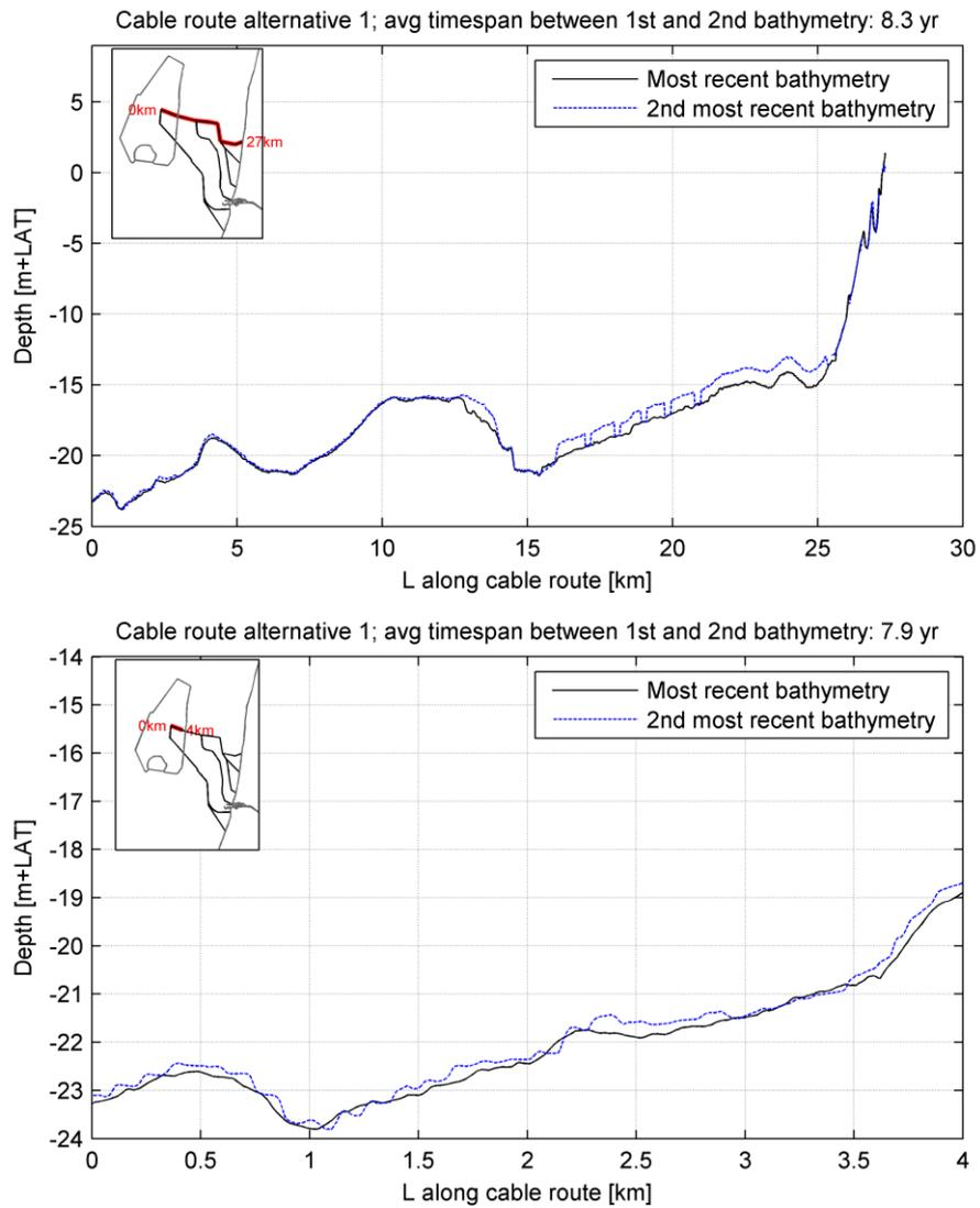
Figure 2.5 Example plot of bathymetry along cable route alternative 1. Top panel: full route, bottom panel: stretch of 4 km.
