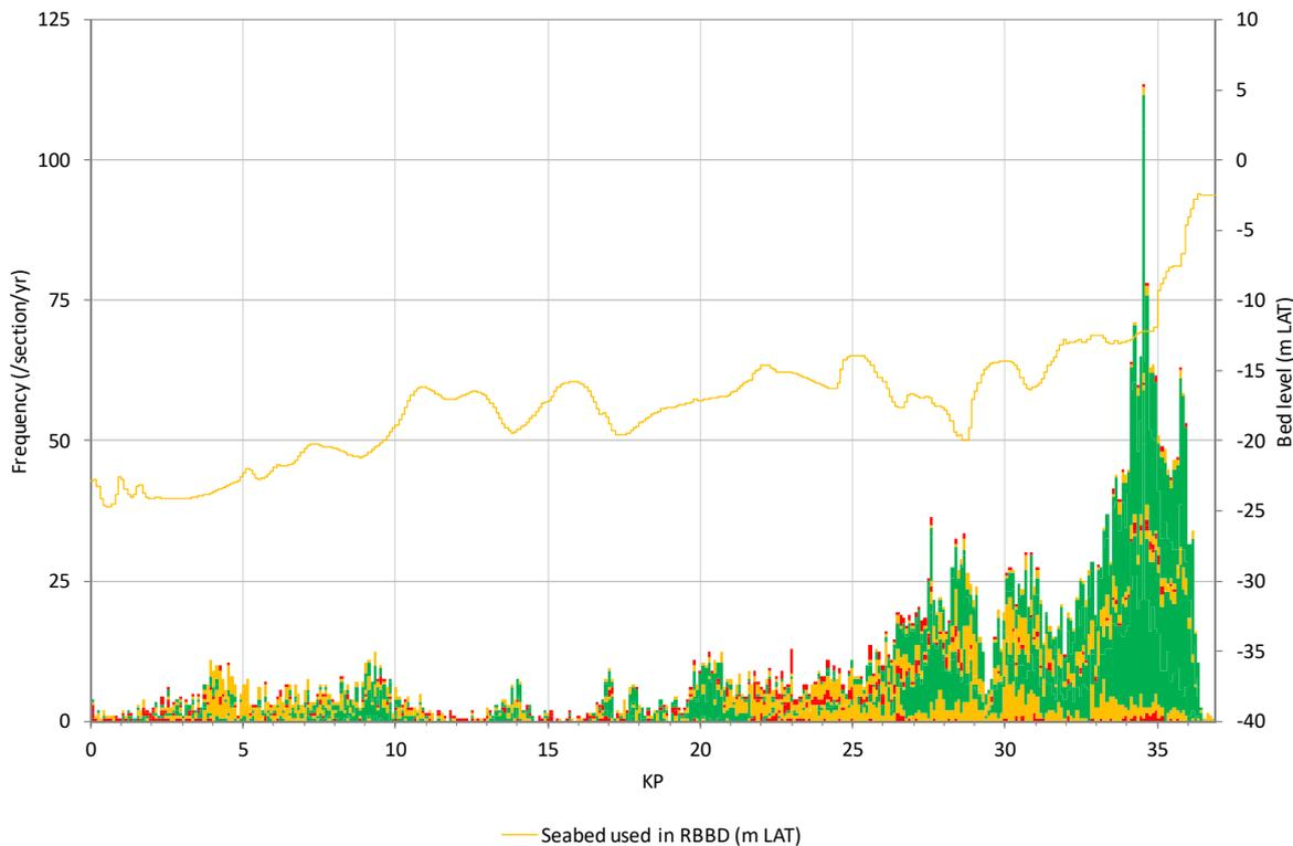
**Figure 5.16** Frequency that fishing activities interacting with Hollandse Kust (noord) route alternative 6. The colours are explained in the next paragraph.
