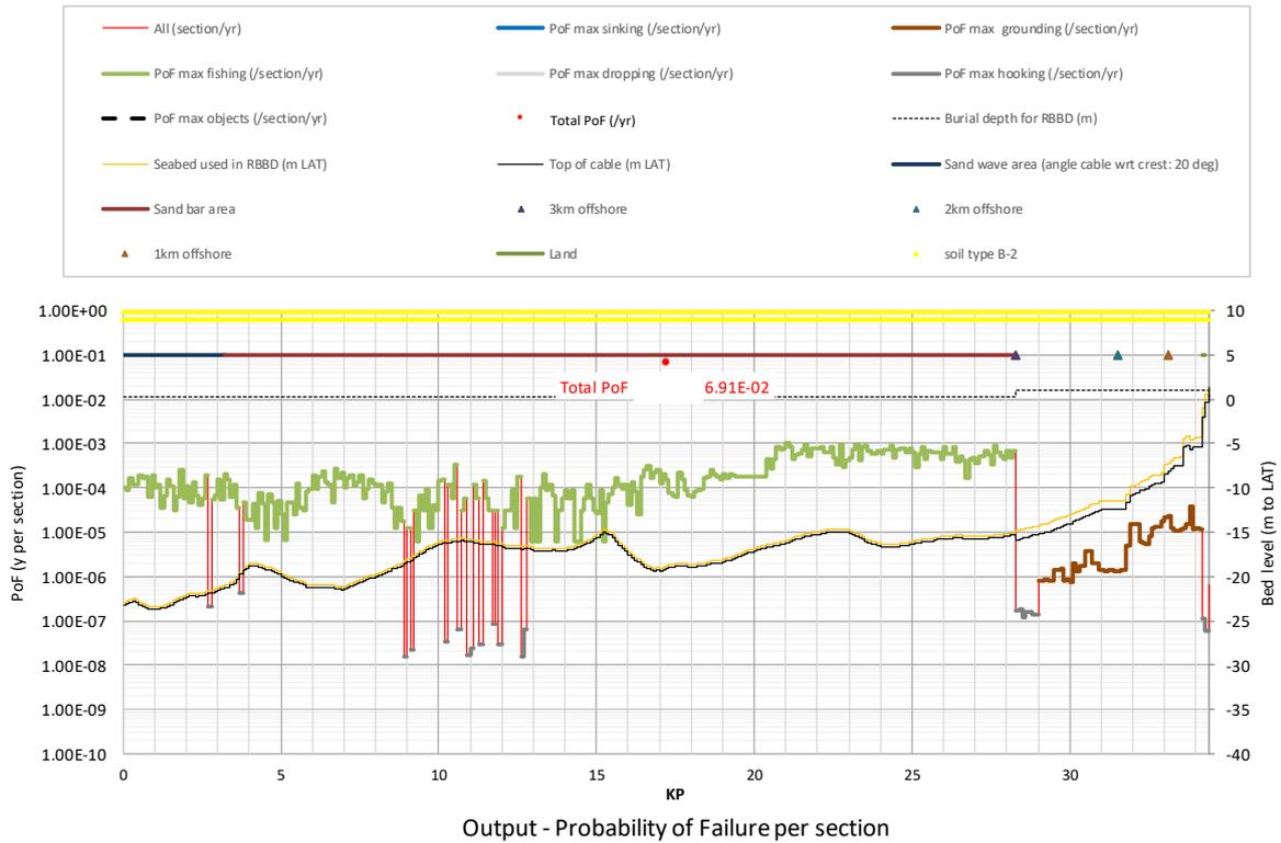
**Figure A2.51** Probability of Failure (PoF) for **Hollandse Kust (noord) route alternative 3**: Minimum scenario = burial scenario 2 + pre-sweeping, burial depth is 1 m (nearshore, < 3km from shore), 0.3 m (offshore, > 3km)
