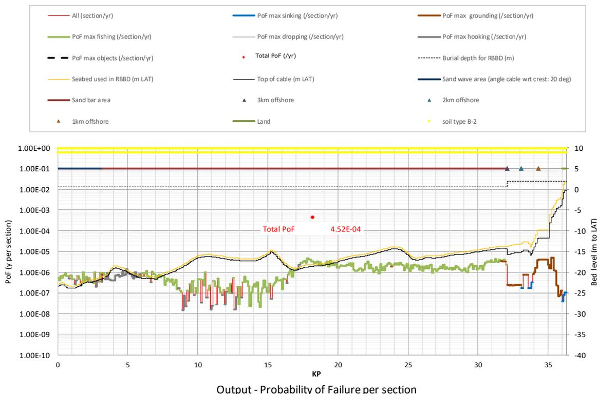
Figure 7.2 Probability of Failure (PoF) for Hollandse Kust (noord) route alternative 4: Signal scenario: Burial depth is 2 m (KP>32.1), 0.5 m (KP<32.1).
