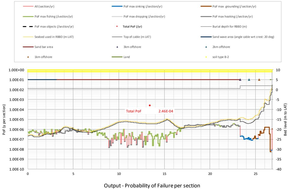
**Figure A2.43** Probability of Failure (PoF) for *Hollandse Kust (noord)* route alternative 1: Signal scenario = burial scenario 1 + pre-sweeping, burial depth is 2 m (nearshore, < 3km from shore), 0.5 m (offshore, > 3km)
