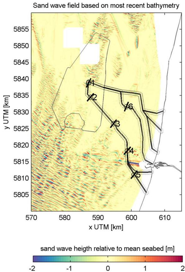
Figure 2.9 Location six transects for sand wave Fourier analysis
