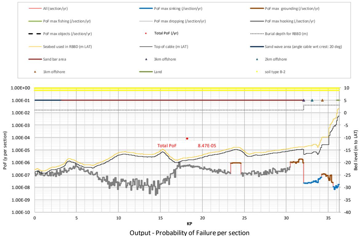
**Figure A2.40** Probability of Failure (PoF) for *Hollandse Kust (noord)* route alternative 4 and 5: Installation scenario = Initial permitting requirements + pre-sweeping, burial depth is 3 m (nearshore, < 3km from shore), 1 m (offshore, > 3km)
