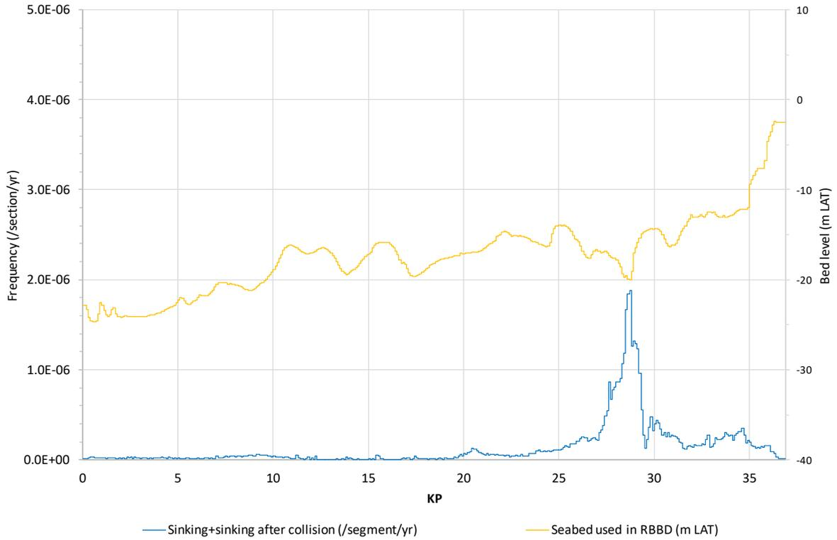
**Figure A2.11** Frequency that critical ship sinking occurs on **Hollandse Kust (noord) route alternative 6**. Note: The scale of the y-axis is a factor 10 larger compared to routes 1-5.
