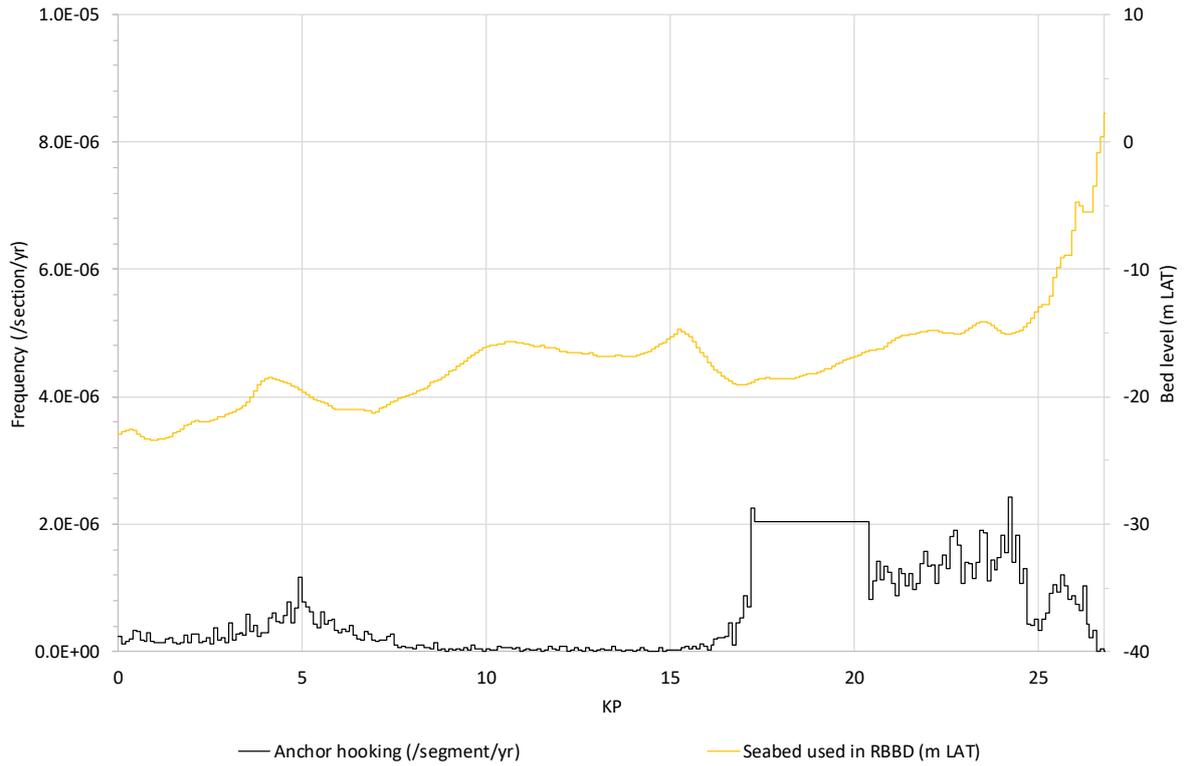
**Figure A2.25** Frequency that critical anchor hooking occurs on *Hollandse Kust (noord)* route alternative 1.
