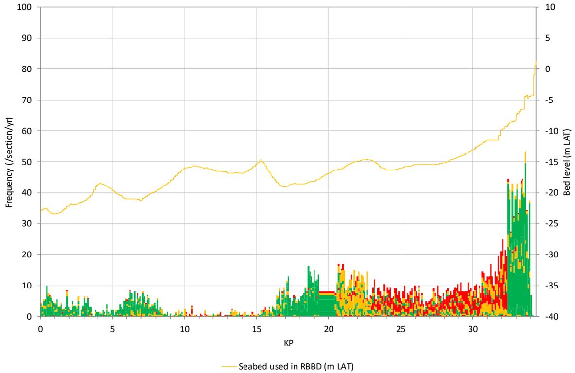
**Figure A2.33** Frequency that fishing activities interacting with *Hollandse Kust (noord)* route alternative 3.
