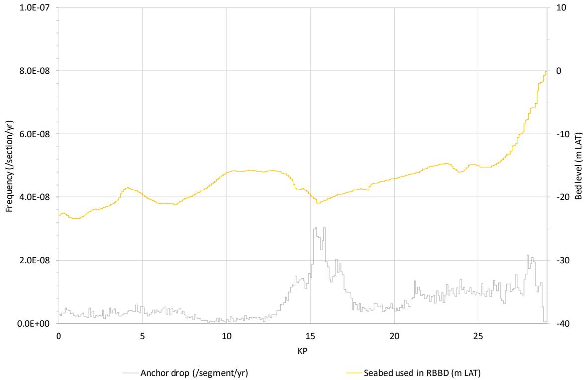
**Figure 5.8** Frequency that critical anchor dropping occurs on Hollandse Kust (noord) route alternative 2.
