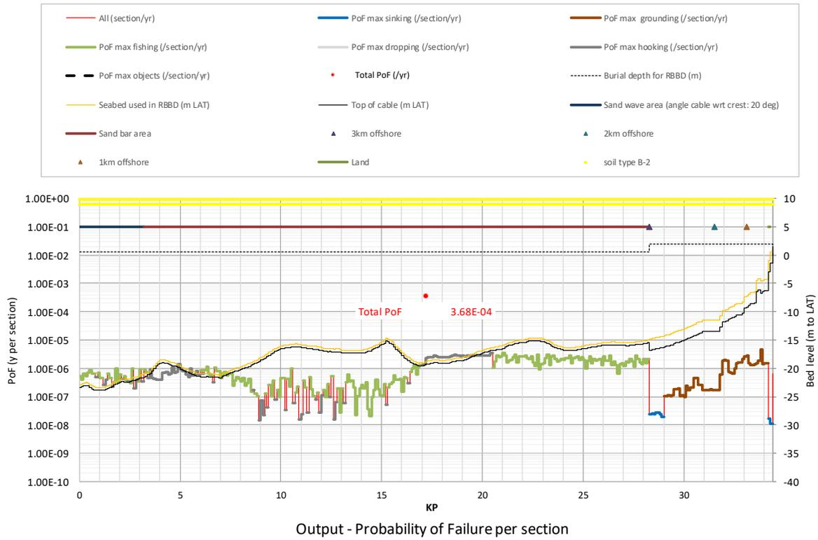
**Figure A2.45** Probability of Failure (PoF) for *Hollandse Kust (noord)* route alternative 3: Signal scenario = burial scenario 1 + pre-sweeping, burial depth is 2 m (nearshore, < 3km from shore), 0.5 m (offshore, > 3km)
