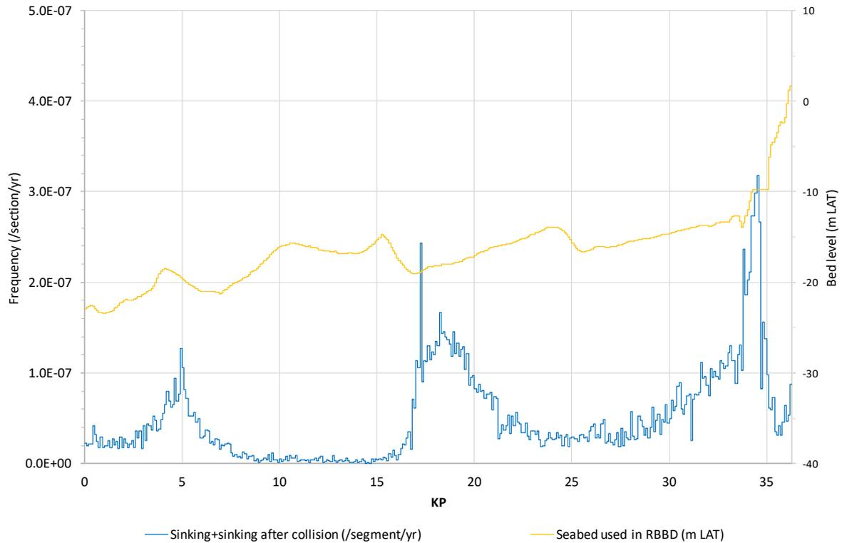
**Figure A2.10** Frequency that critical ship sinking occurs on *Hollandse Kust (noord) route alternative 4 and 5*.
