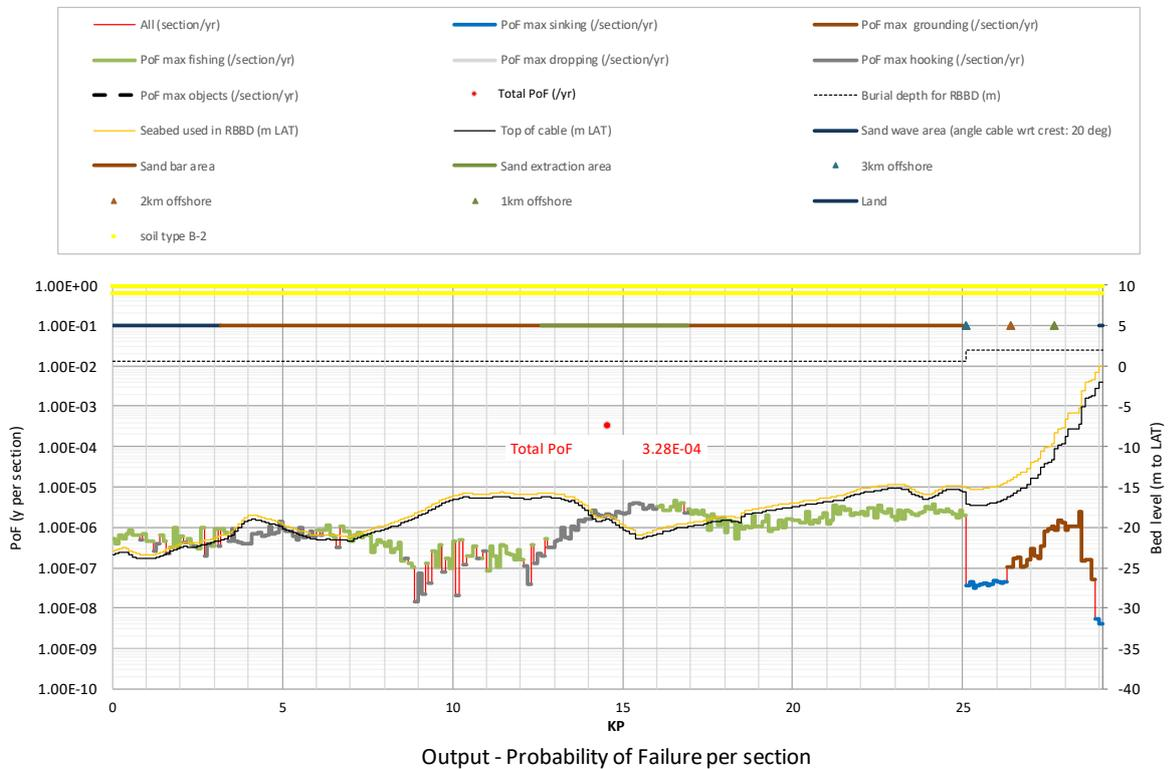
**Figure A2.44** Probability of Failure (PoF) for *Hollandse Kust (noord)* route alternative 2: Signal scenario = burial scenario 1 + pre-sweeping, burial depth is 2 m (nearshore, < 3km from shore), 0.5 m (offshore, > 3km)
