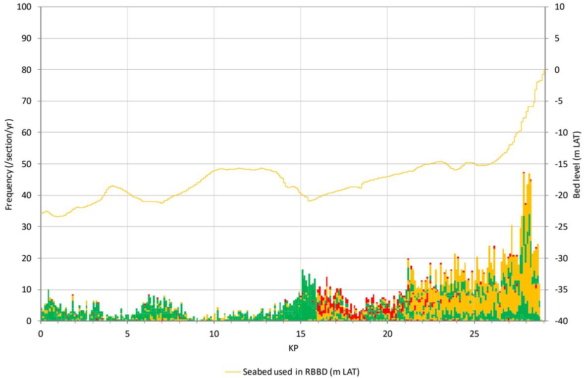
**Figure 5.14** Frequency that fishing activities interacting with Hollandse Kust (noord) route alternative 2. The colours are explained in the next paragraph.
