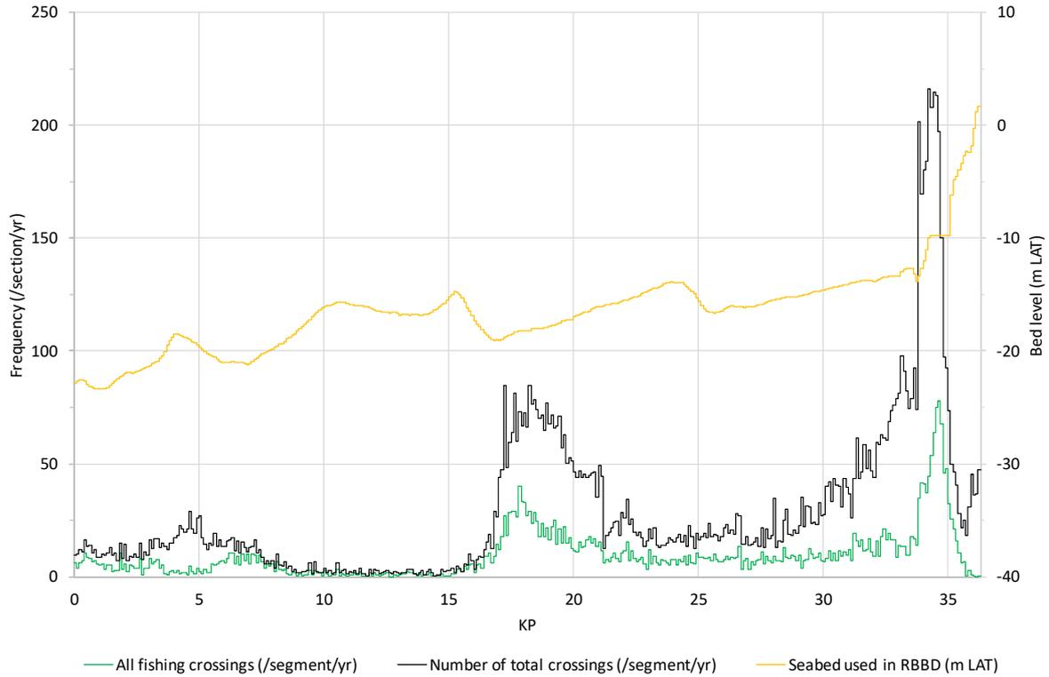
**Figure 5.2** Frequency of all the ships (black line) and fishing ships (green line) that cross route alternative 4 and 5 (/section/yr) as function of the cable route (KP). The numbers are based on two year of AIS data (from 1 January 2015 to 31 December 2016) for each segment of ~100 m. The seabed level (yellow line) that is used for the RBBB is presented in order to link the AIS data to the water depth.
