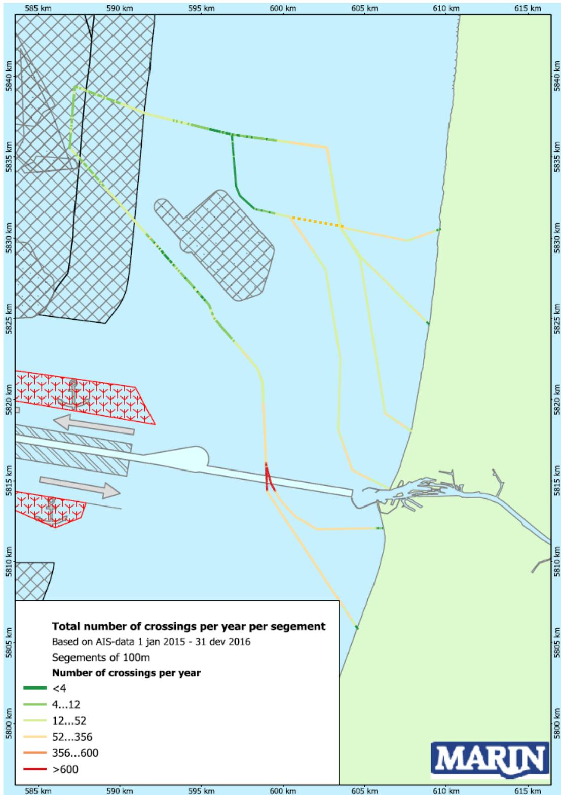
**Figure 2.2** Total passages per 100 m segment per year over all route alternatives based on AIS data from 1 January 2015 – 31 December 2016, coloured by shipping intensity. (Figure 4-3 from Marin report included as Annex 1). With reference to Figure 1.1 and the accompanying Note, the updated routes are indicated by the broken connecting line in above Figure. The crossing frequencies for this new segment have been derived from the crossing frequencies and is further explained in Annex 1.
