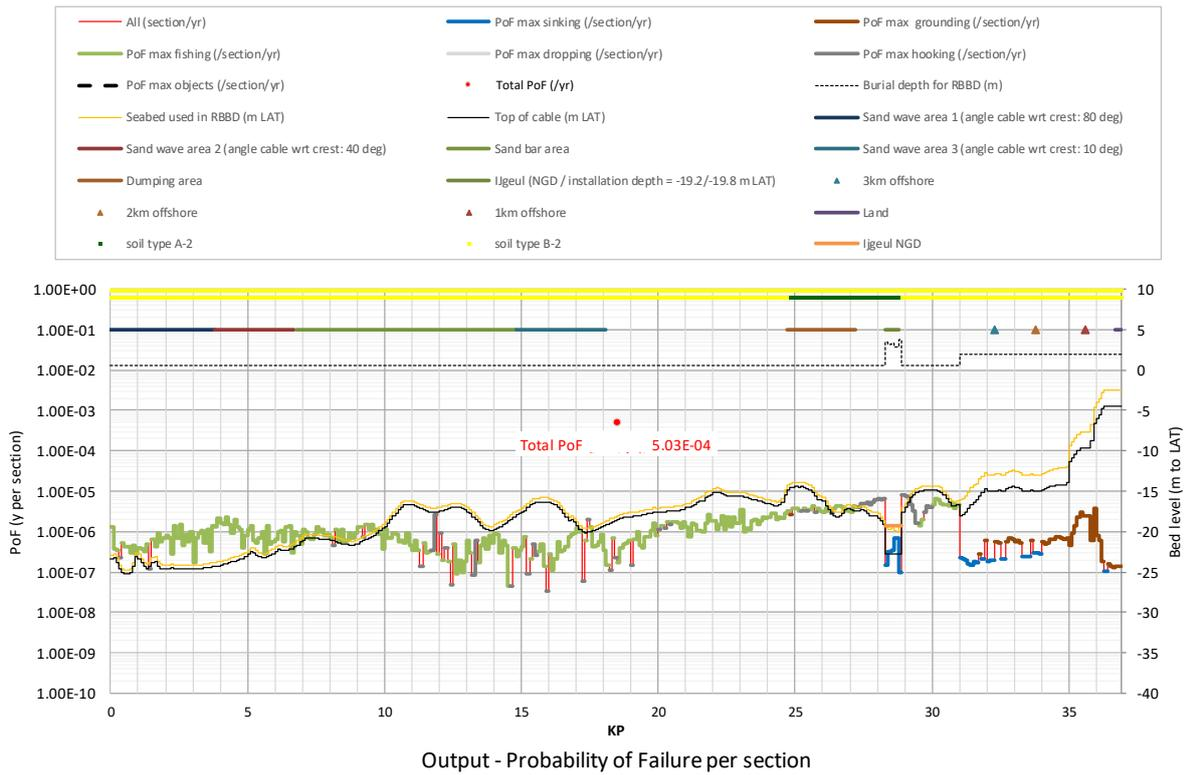
**Figure A2.47** Probability of Failure (PoF) for *Hollandse Kust (noord)* route alternative 6: Signal scenario = burial scenario 1 + pre-sweeping, burial depth is 2 m (nearshore, < 3km from shore), 0.5 m (offshore, > 3km), burial in IJ-geul 3m below -19.8 m LAT (= NGD-0.5m)
