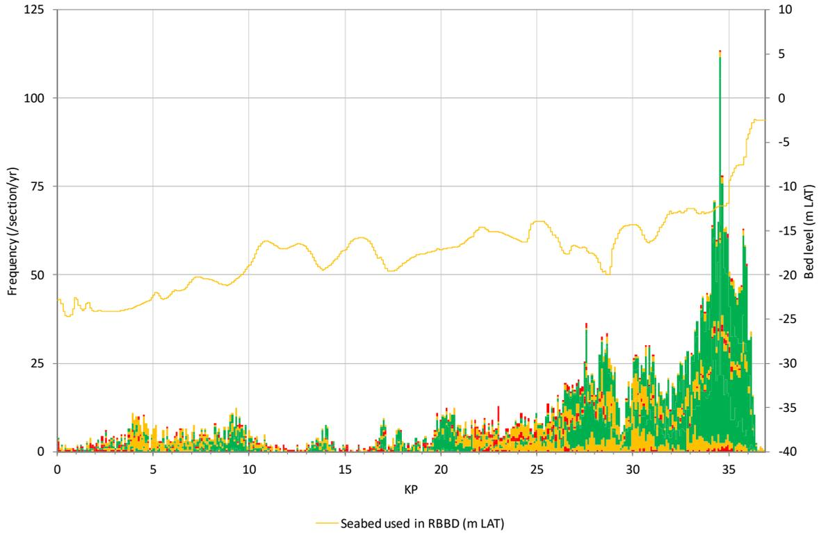
**Figure A2.35** Frequency that fishing activities interacting with *Hollandse Kust (noord)* route alternative 6.
