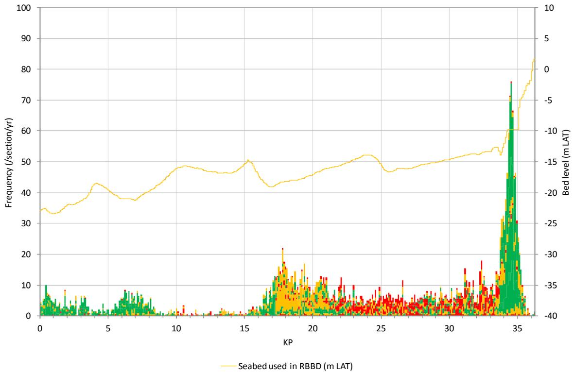
**Figure 5.15** Frequency that fishing activities interacting with Hollandse Kust (noord) route alternative 4. The colours are explained in the next paragraph.
