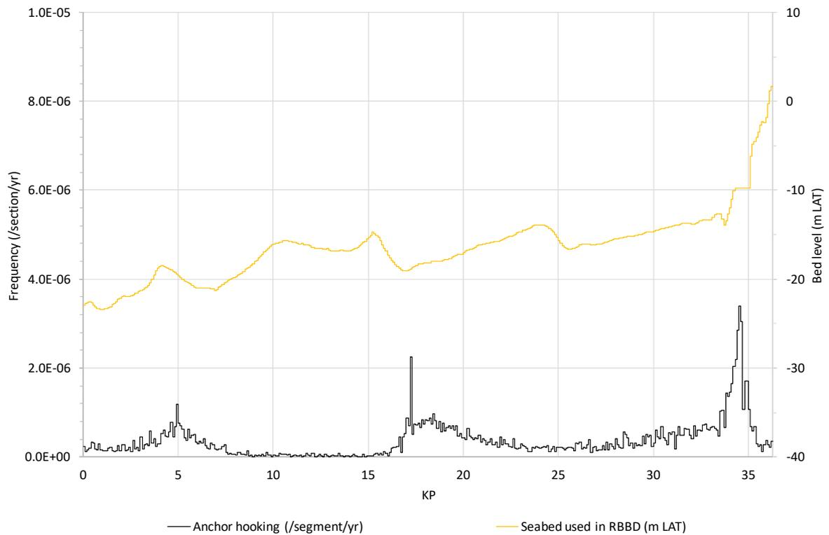
**Figure A2.28** Frequency that critical anchor hooking occurs on *Hollandse Kust (noord)* route alternative 4 and 5.
