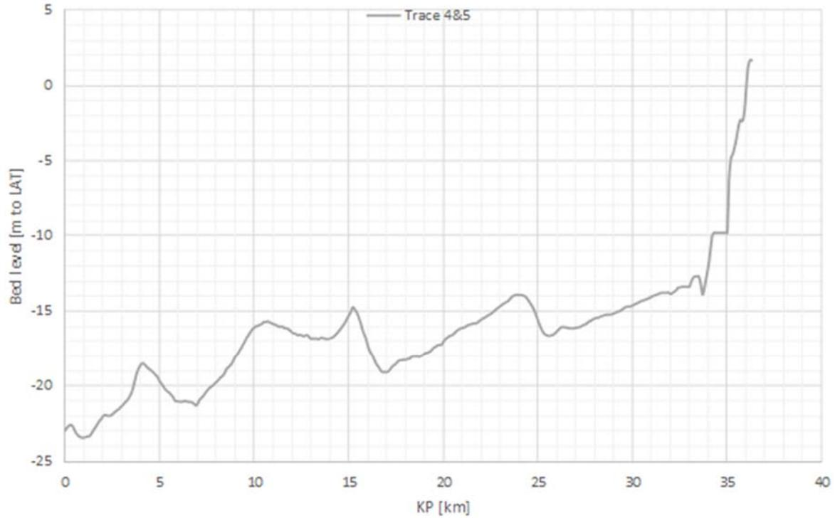
**Figure 3.2** *Sea bed (in m relative to LAT) along the Hollandse Kust (noord) export cables route alternatives 4 and 5 (offshore part only) (/7/).*
