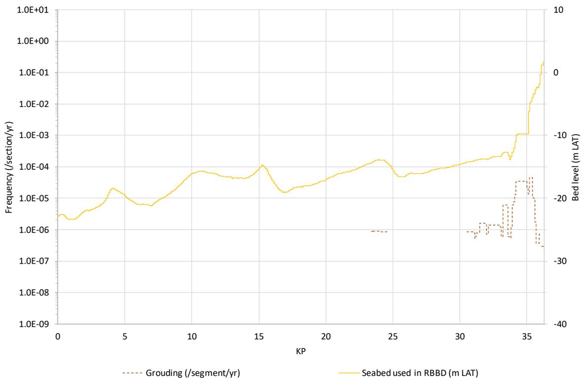
**Figure 5.6** Frequency that critical ship grounding occurs on Hollandse Kust (noord) route alternative 4.
