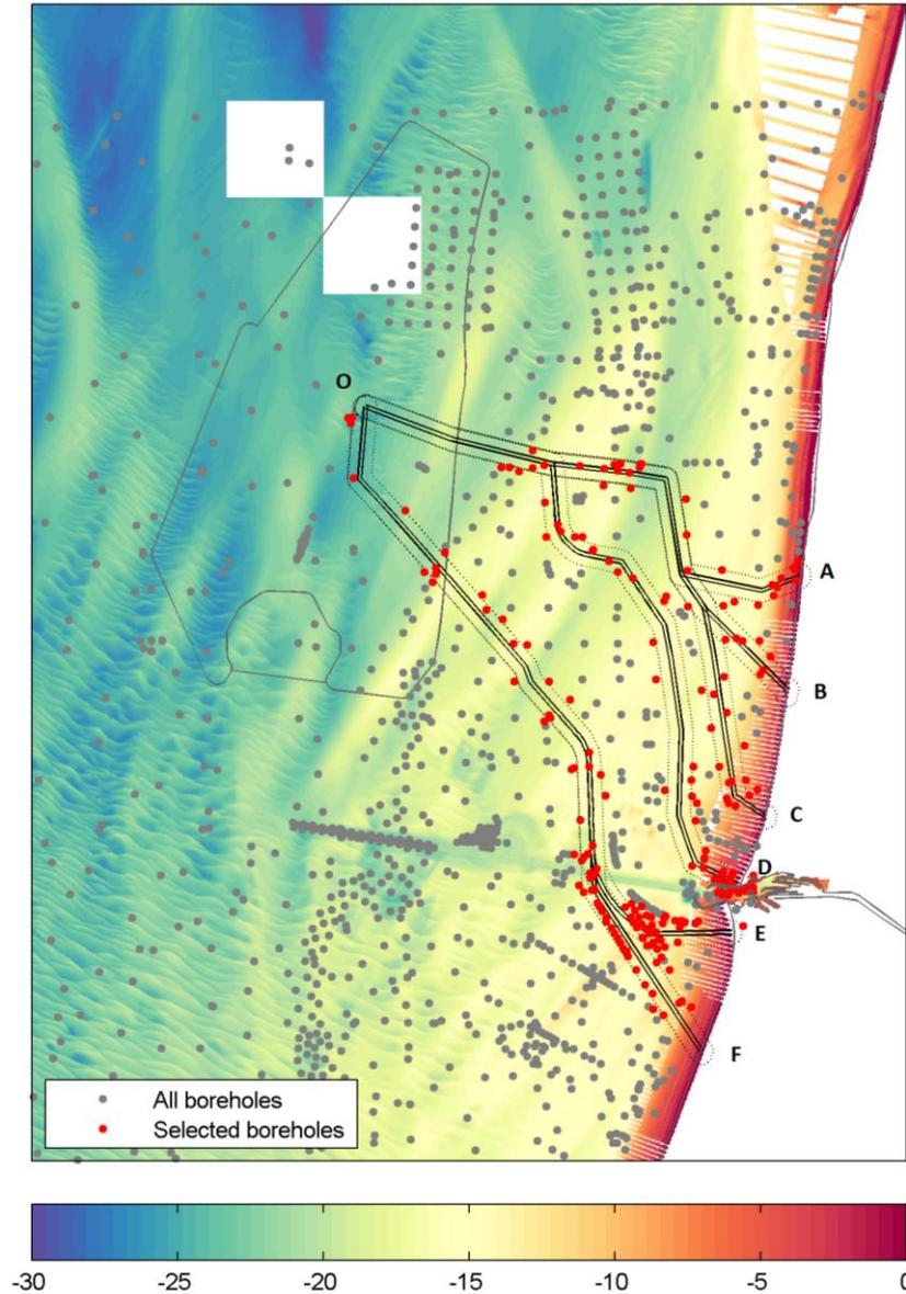
Figure 5.3: Borehole locations (DINO loket) against bathymetry and route alternatives.
