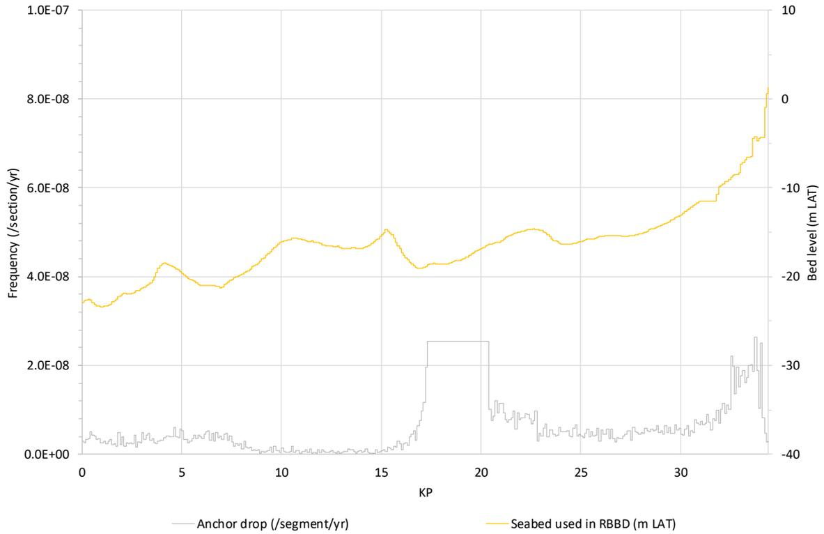
**Figure A2.21** Frequency that critical anchor dropping occurs on *Hollandse Kust (noord)* route alternative 3.
