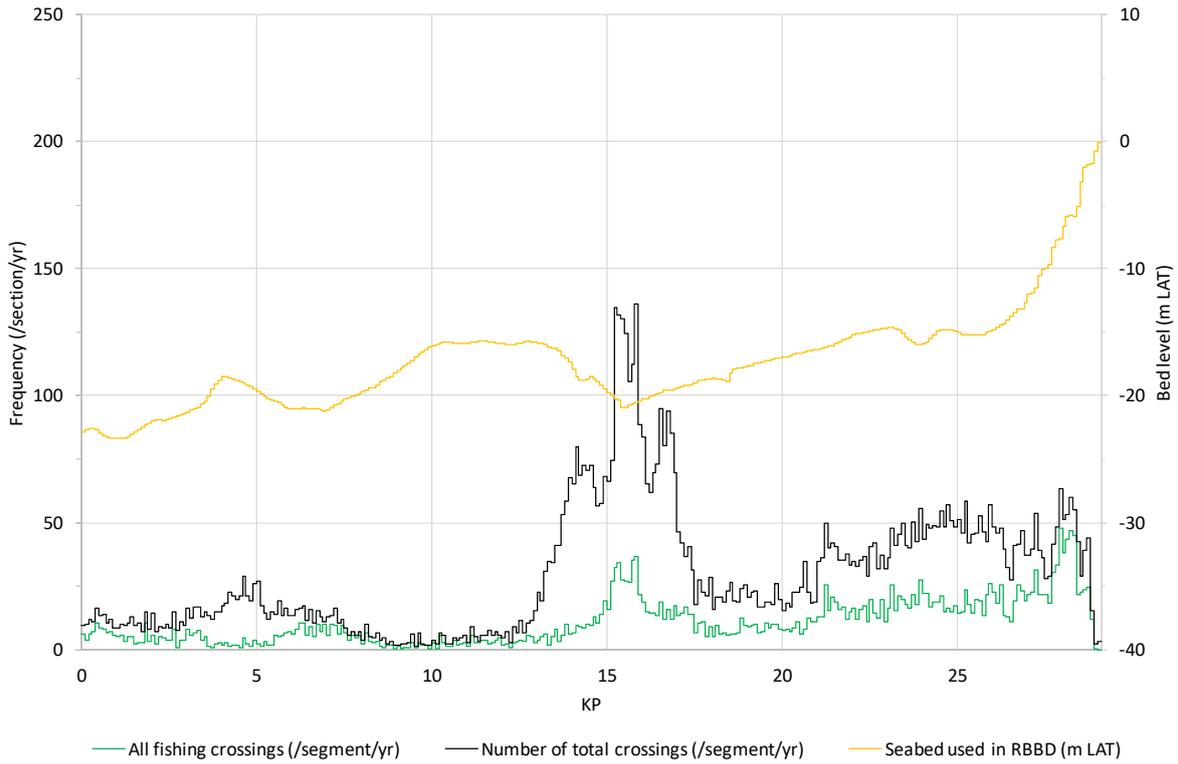
**Figure 5.1** Frequency of all the ships (black line) and fishing ships (green line) that cross route alternative 2 (/section/yr) as function of the cable route (KP). The numbers are based on two year of AIS data (from 1 January 2015 to 31 December 2016) for each segment of ~100 m. The seabed level (yellow line) that is used for the RBBB is presented in order to link the AIS data to the water depth.
