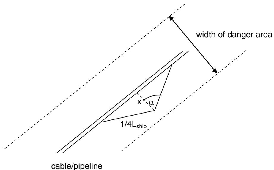
Figure 3 Danger area for hooking the pipeline
