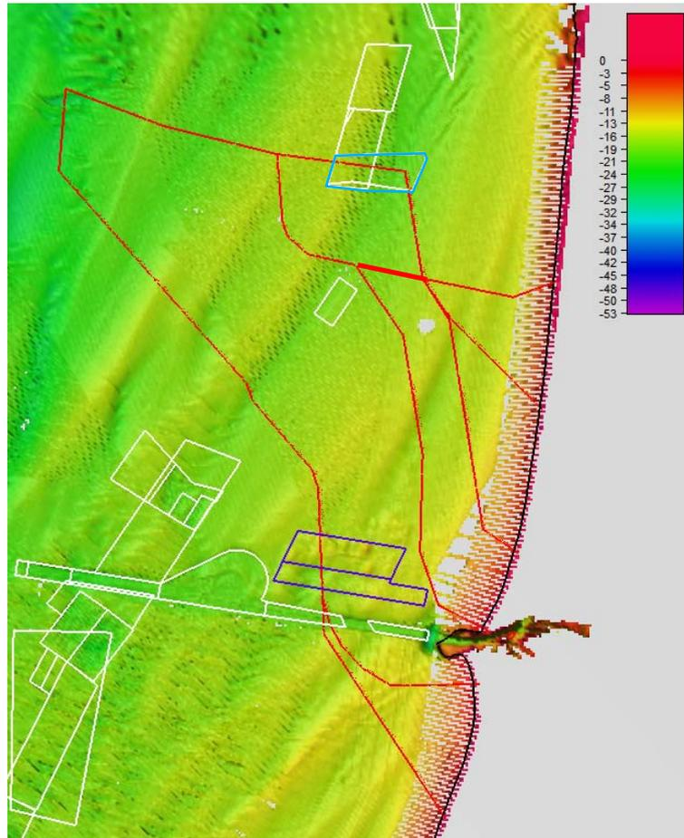
**Figure 4.2** Overview of cable routes (red) and the spoil dumping area (outlined purple) and a sand extraction area (outlined blue).
