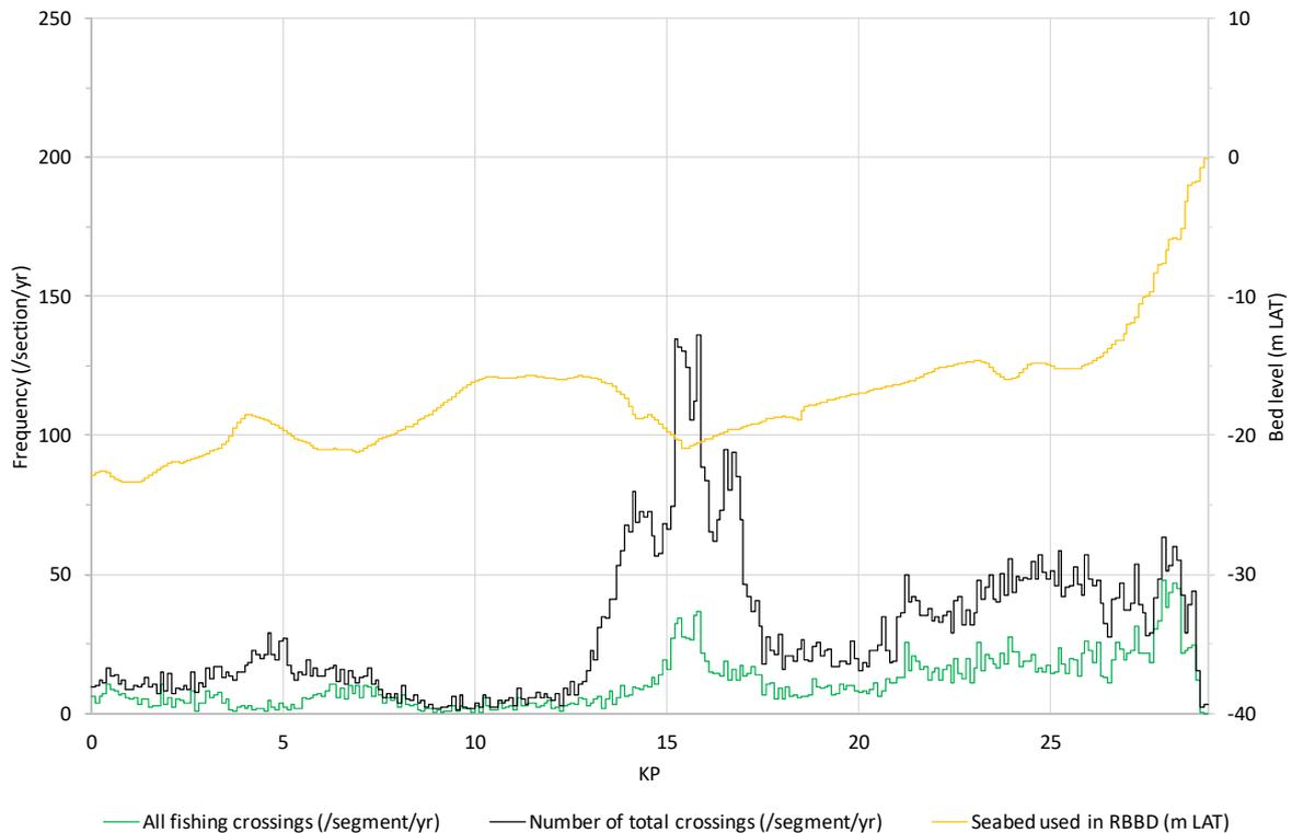
**Figure A2.2** Frequency of all the ships (black line) and fishing ships (green line) that cross **Hollandse Kust (noord) route alternative 2** (/segment/yr) as function of the cable route (KP).
