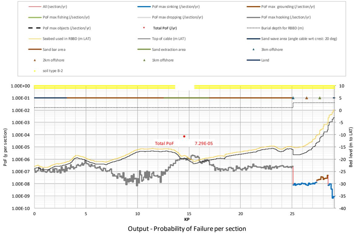
**Figure A2.38** *Probability of Failure (PoF) for Hollandse Kust (noord) route alternative 2: Installation scenario = Initial permitting requirements + pre-sweeping, burial depth is 3 m (nearshore, < 3km from shore), 1 m (offshore, > 3km)*
