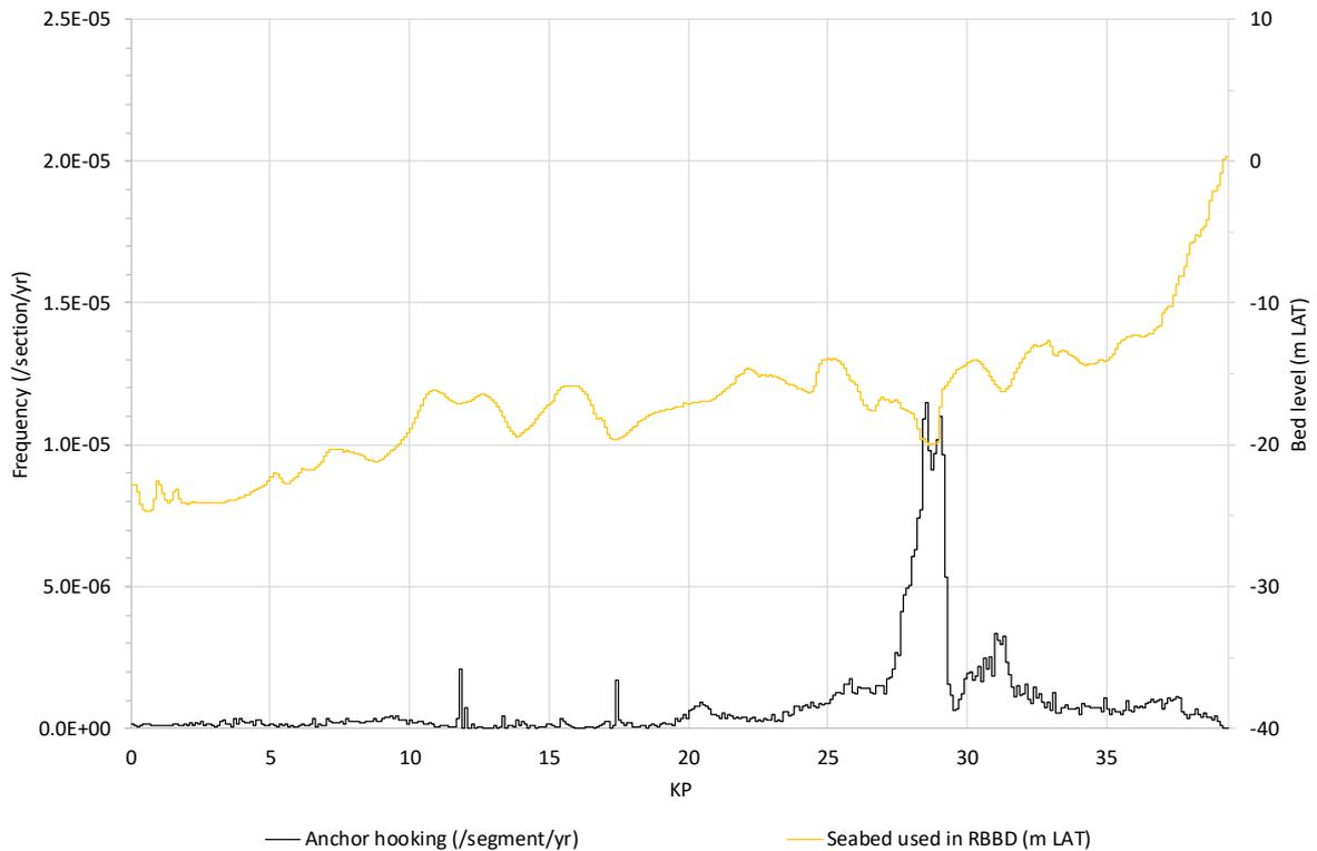
**Figure A2.30** Frequency that critical anchor hooking occurs on **Hollandse Kust (noord) route alternative 7**. Note: The scale of the y-axis is a factor 2 larger compared to routes 1-5.
