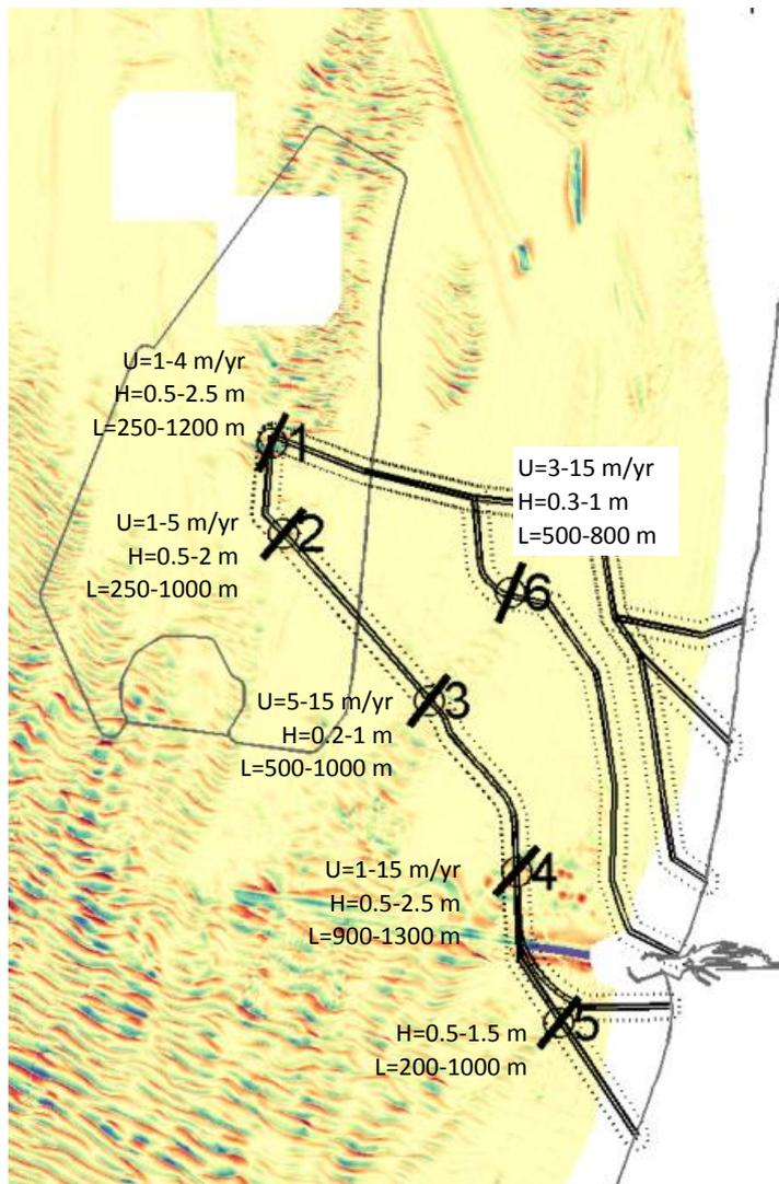
Figure 2.11 Range of sand wave characteristics
