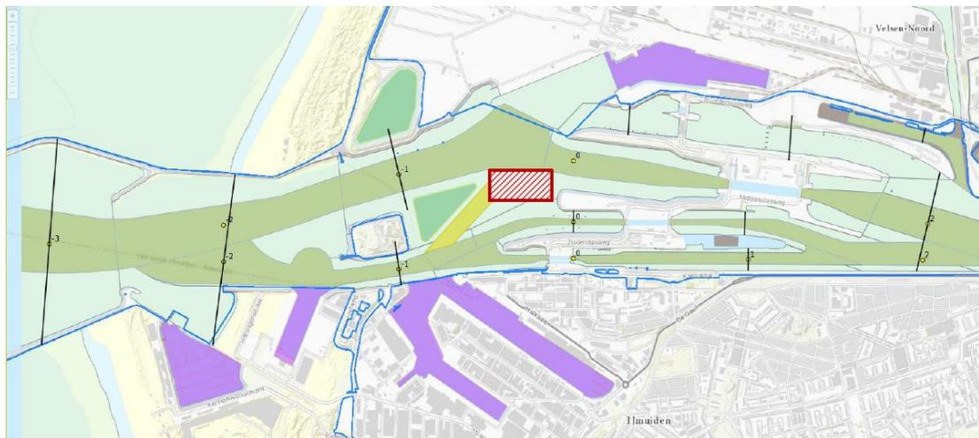
Figure 4.6: Location of Verbindingskanaal, which is crossed by cable route alternative 4 and 5. The configuration of this channel will be changed as a result of the New Sea Lock, but how is not determined yet. (Waterboekje, Rijkswaterstaat)
