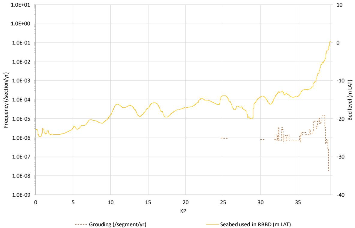
**Figure A2.18** Frequency that critical ship grounding occurs on **Hollandse Kust (noord)** route alternative 7.
