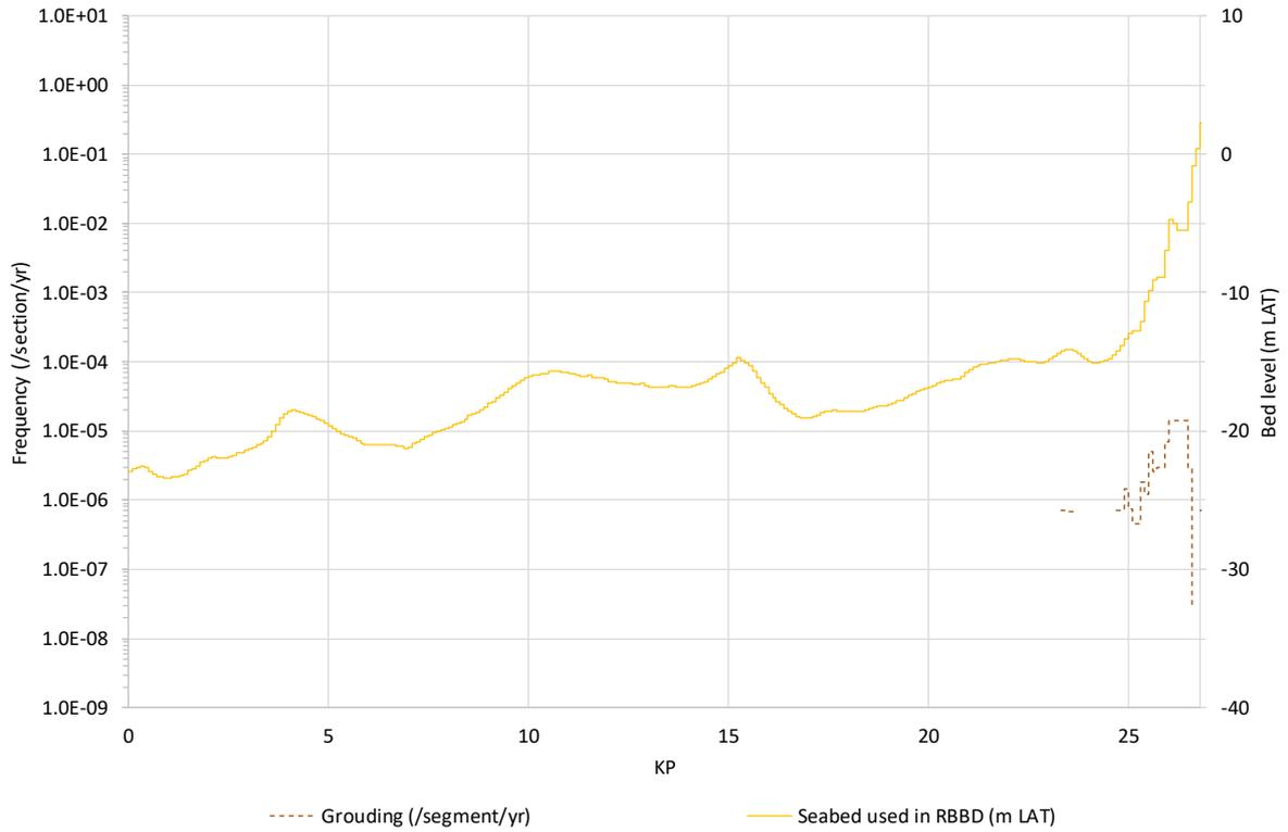
**Figure A2.13** Frequency that critical ship grounding occurs on *Hollandse Kust (noord)* route alternative 1.
