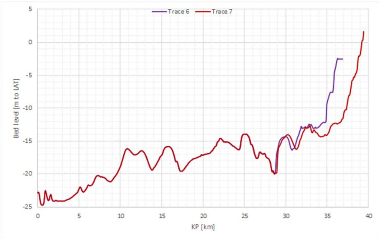
**Figure 3.3** Sea bed (in m relative to LAT) along the Hollandse Kust (noord) export cables route alternatives 6 and 7 (/7/).
