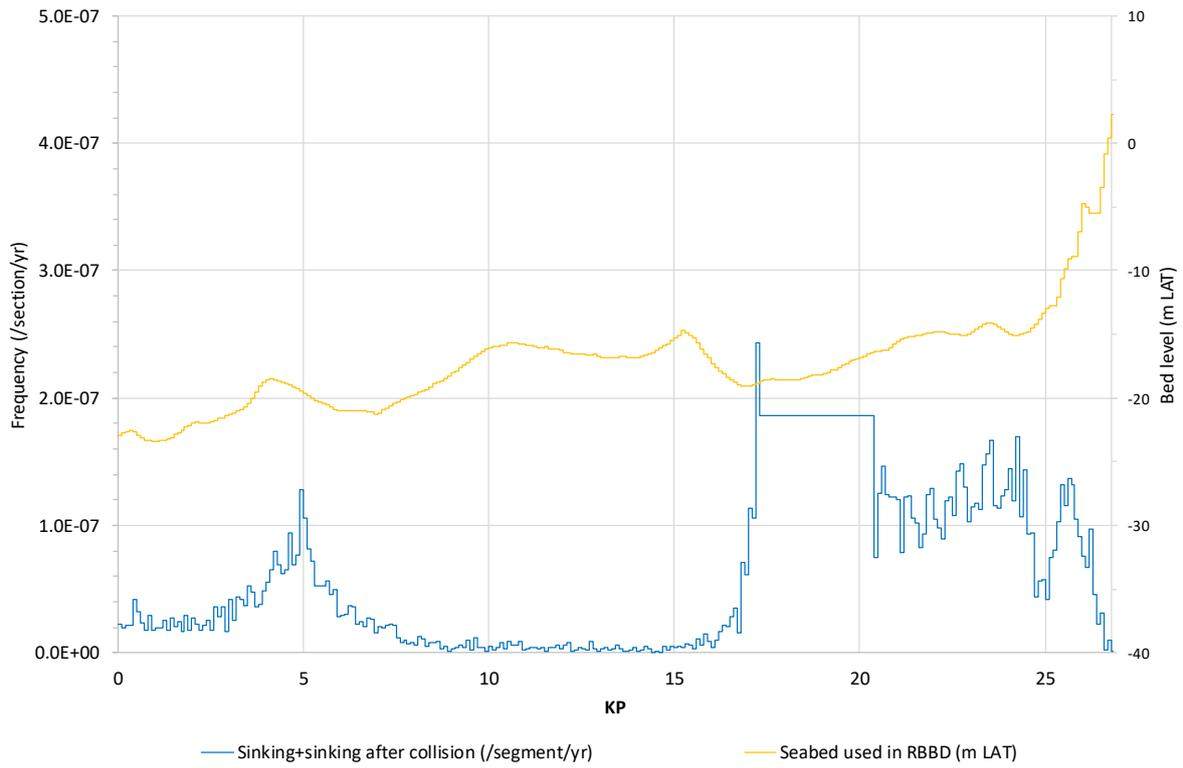
**Figure A2.7** Frequency that critical ship sinking occurs on **Hollandse Kust (noord) route alternative 1.**
