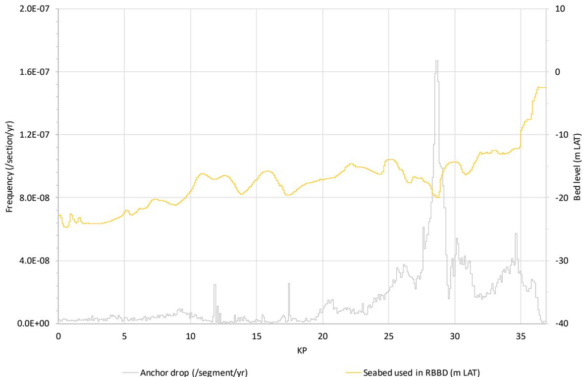
**Figure A2.23** Frequency that critical anchor dropping occurs on **Hollandse Kust (noord) route alternative 6**. Note: The scale of the y-axis is a factor 2 larger compared to routes 1-5.
