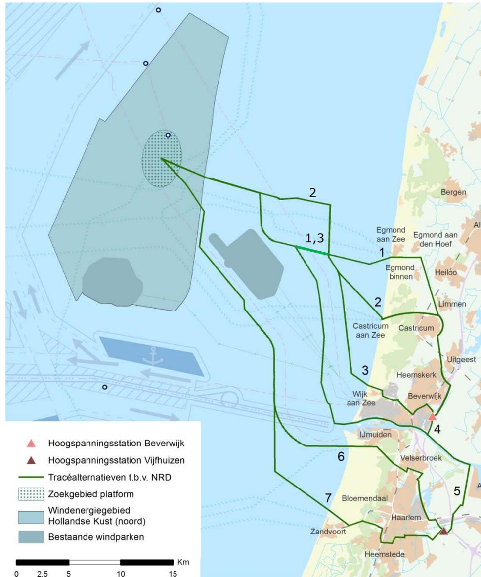
**Figure 1.1** Export cables Hollandse Kust (noord); all seven cable route alternatives are shown;
