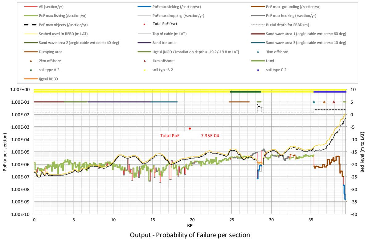
**Figure A2.48** Probability of Failure (PoF) for *Hollandse Kust (noord)* route alternative 7: Signal scenario = burial scenario 1 + pre-sweeping, burial depth is 2 m (nearshore, < 3km from shore), 0.5 m (offshore, > 3km), burial in IJ-geul 3m below -19.8 m LAT (= NGD-0.5m)
