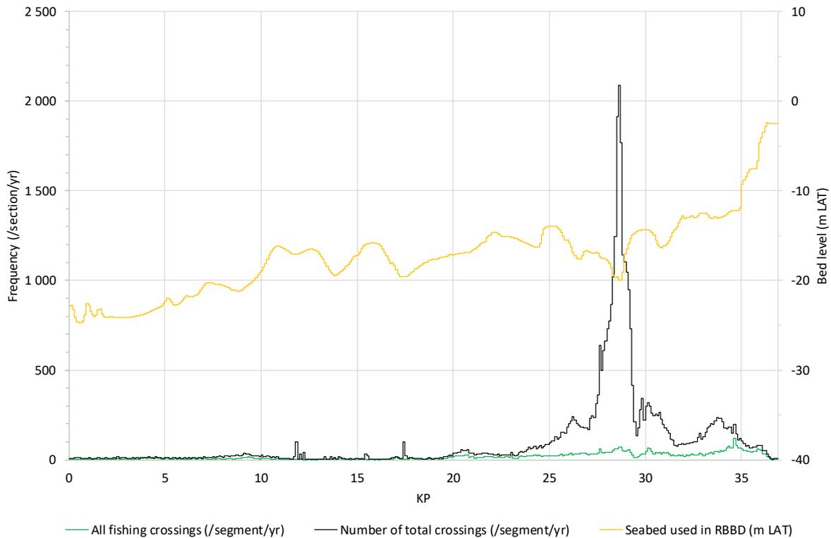
**Figure 5.3** Frequency of all the ships (black line) and fishing ships (green line) that cross
