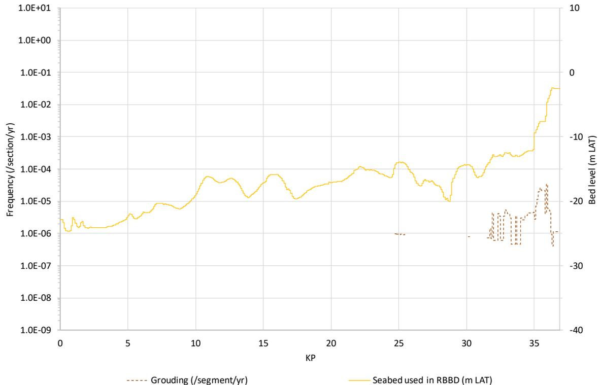
**Figure 5.7** Frequency that critical ship grounding occurs on Hollandse Kust (noord) route alternative 6.
