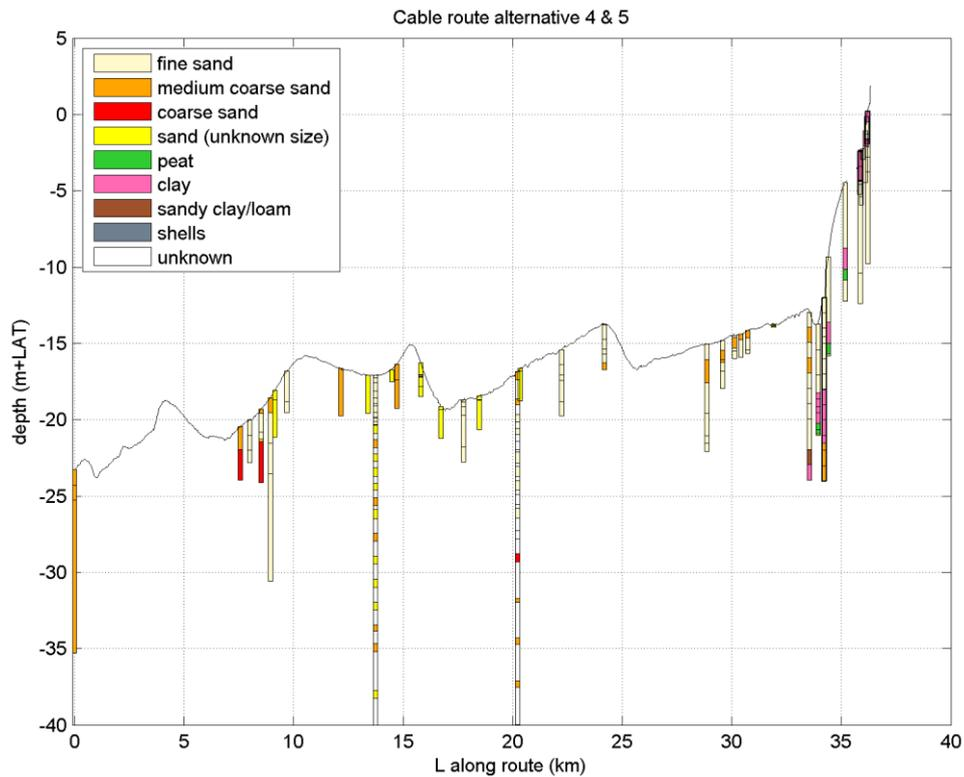
Figure 5.7: Bathymetric and borehole cross-section from O-C, showing mainly medium sand at the surface. Near shore coarse sand at the surface and clay of the Layer of Velsen (part of the Naaldwijk formation) is apparent at the surface and at 8m depth, covering peat beds from the Nieuwkoop formation.
