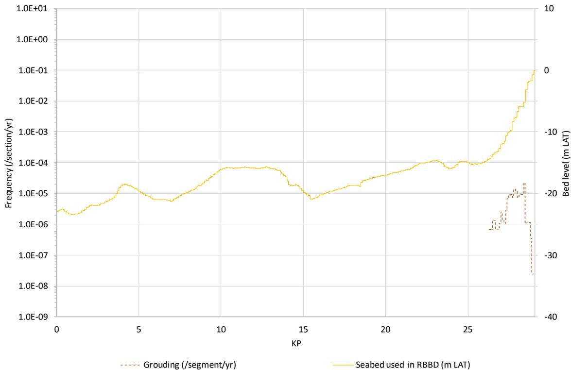
**Figure 5.5** Frequency that critical ship grounding occurs on Hollandse Kust (noord) route alternative 2.
