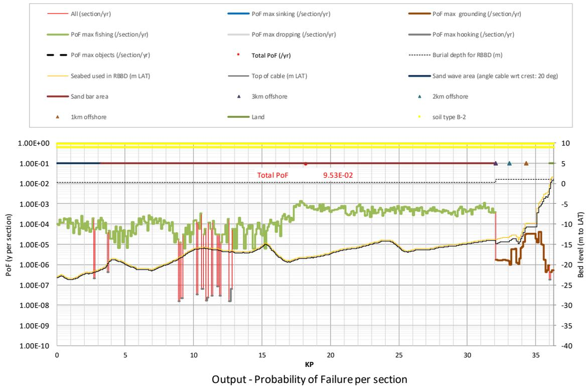
**Figure A2.52** Probability of Failure (PoF) for **Hollandse Kust (noord) route alternative 4 and 5**: Minimum scenario = burial scenario 2 + pre-sweeping, burial depth is 1 m (nearshore, < 3km from shore), 0.3 m (offshore, > 3km)
