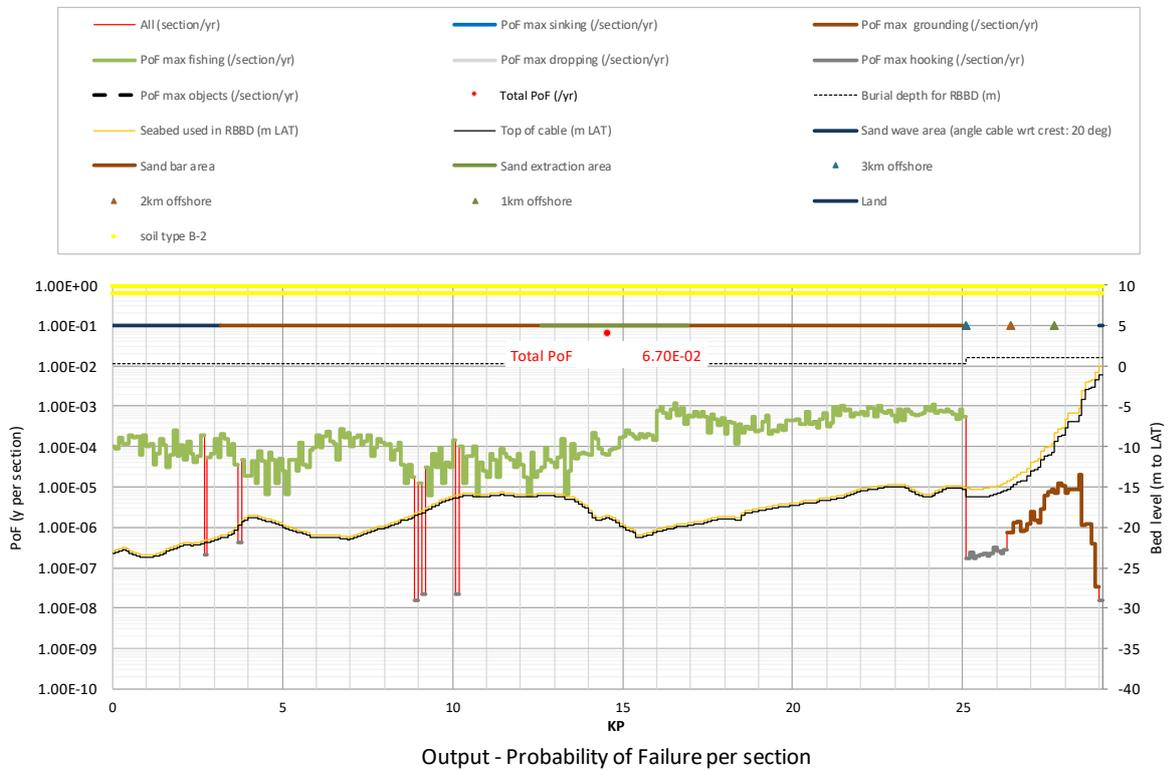
**Figure A2.50** Probability of Failure (PoF) for *Hollandse Kust (noord)* route alternative 2: Minimum scenario = burial scenario 2 + pre-sweeping, burial depth is 1 m (nearshore, < 3km from shore), 0.3 m (offshore, > 3km)
