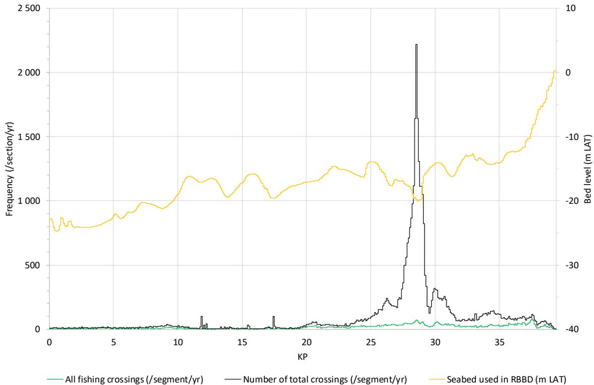
**Figure A2.6** Frequency of all the ships (black line) and fishing ships (green line) that cross **Hollandse Kust (noord) route alternative 7** (/section/yr) as function of the cable route (KP). Note: The scale of the y-axis is a factor 10 larger compared to routes 1-5.
