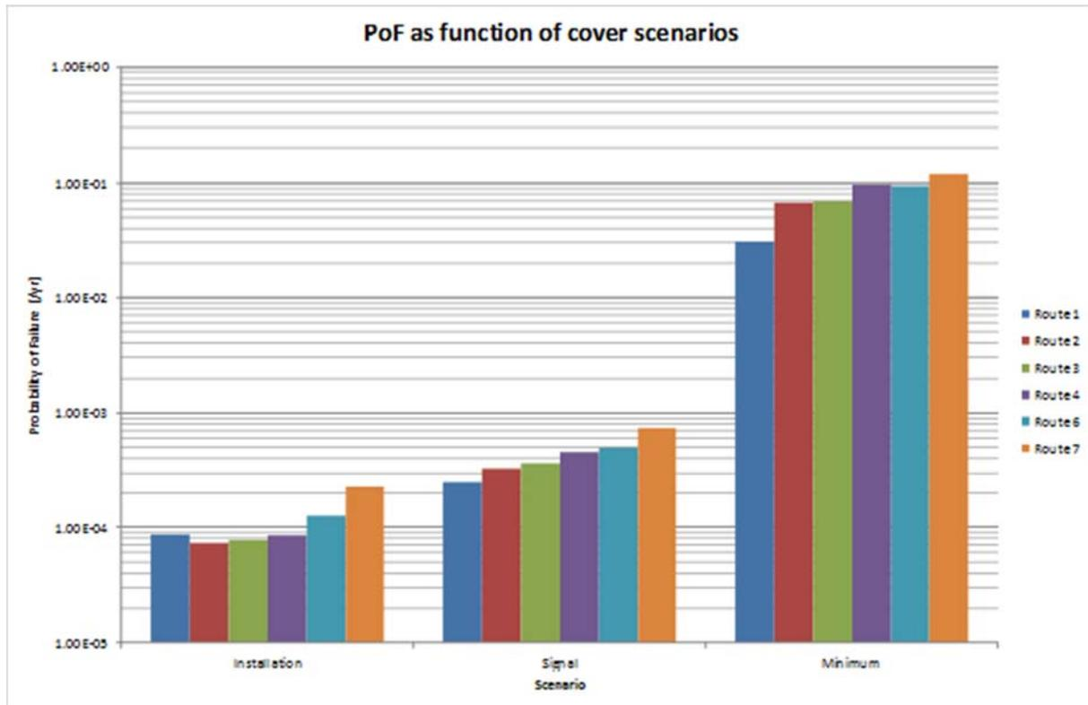
**Figure 7.4** Probability of Failure (PoF) for all Hollandse Kust (noord) route alternatives and all scenarios.
