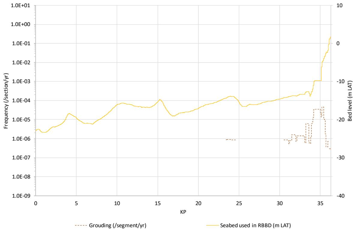
**Figure A2.16** Frequency that critical ship grounding occurs on *Hollandse Kust (noord)* route alternative 4 and 5.
