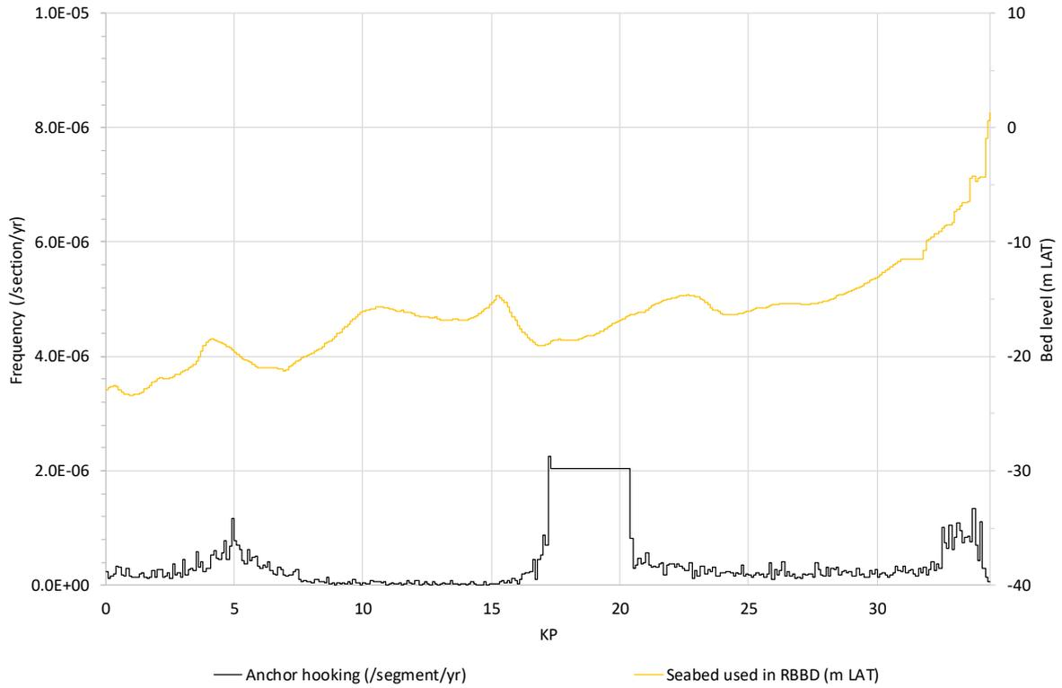
**Figure A2.27** Frequency that critical anchor hooking occurs on *Hollandse Kust (noord)* route alternative 3.
