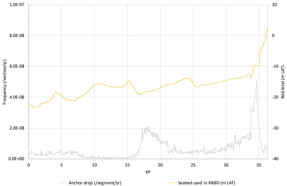
**Figure 5.9** Frequency that critical anchor dropping occurs on Hollandse Kust (noord) route alternative 4.
