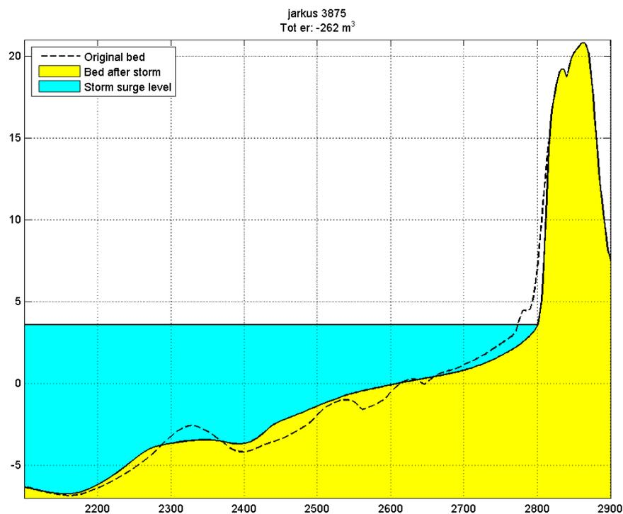
Figure 3.17: Model results of the impact of a 1/100 years storm condition on the most recent recorded coastal profile at landfall location 1.
