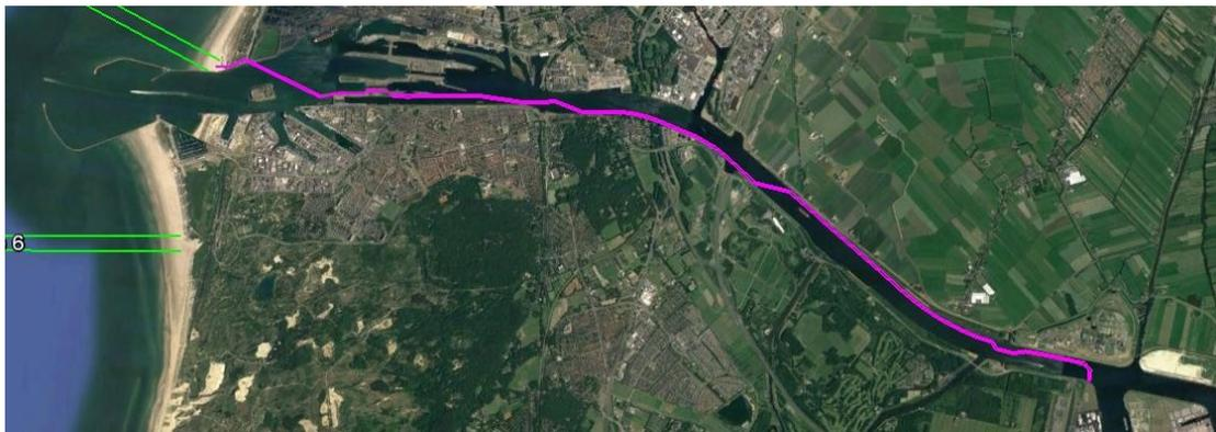
Figure 4.1: Cable route alternative 5 in IJmuiden Port and the Noordzeekanaal (magenta). Alternative 4 follows the same route up to approximately the Wijkertunnel before heading north and reaching land.
