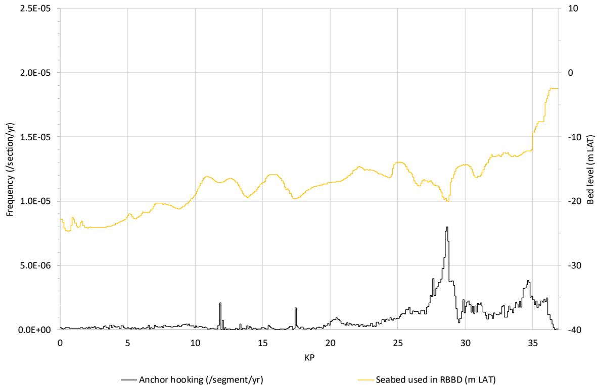
**Figure 5.13** Frequency that critical anchor hooking occurs on Hollandse Kust (noord) route alternative 6.
