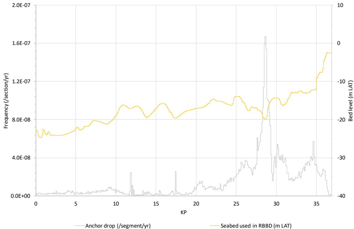
**Figure 5.10** Frequency that critical anchor dropping occurs on Hollandse Kust (noord) route alternative 6.
