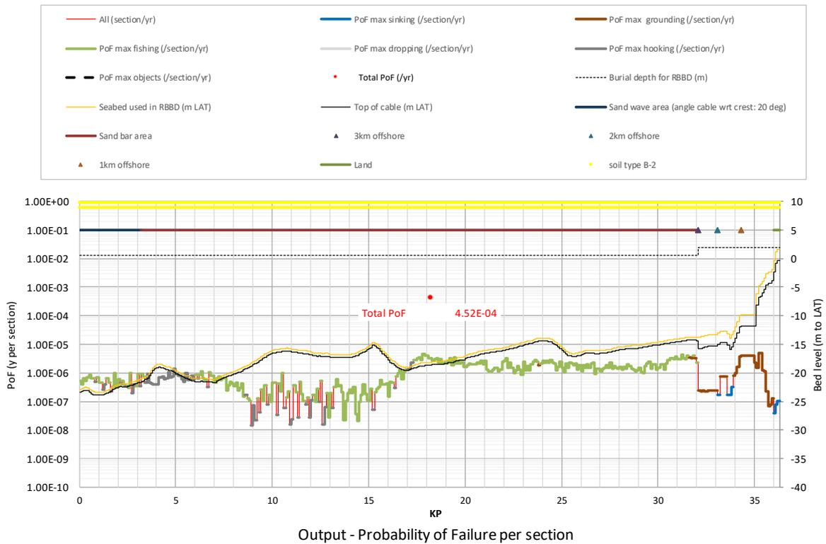
**Figure A2.46** Probability of Failure (PoF) for *Hollandse Kust (noord)* route alternative 4 and 5: Signal scenario = burial scenario 1 + pre-sweeping, burial depth is 2 m (nearshore, < 3km from shore), 0.5 m (offshore, > 3km)
