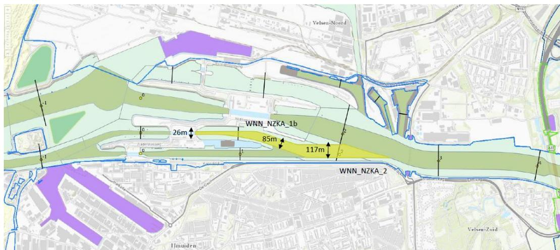
Figure 4.10: Location of Middenbinnentoeleidingskanaal, which is crossed by cable route alternative 4 and 5. The configuration is changed as a result of the New Sea Lock, but not present in the documentation yet. (Waterboekje, Rijkswaterstaat)
