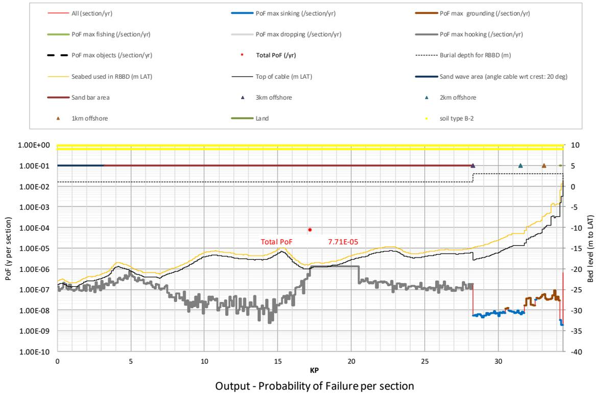
**Figure A2.39** Probability of Failure (PoF) for *Hollandse Kust (noord)* route alternative 3: Installation scenario = Initial permitting requirements + pre-sweeping, burial depth is 3 m (nearshore, < 3km from shore), 1 m (offshore, > 3km)
