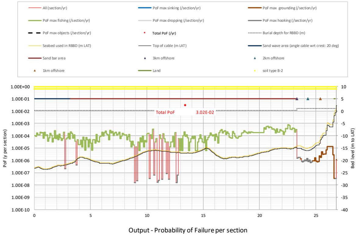
**Figure A2.49** Probability of Failure (PoF) for *Hollandse Kust (noord)* route alternative 1: Minimum scenario = burial scenario 2 + pre-sweeping, burial depth is 1 m (nearshore, < 3km from shore), 0.3 m (offshore, > 3km)
