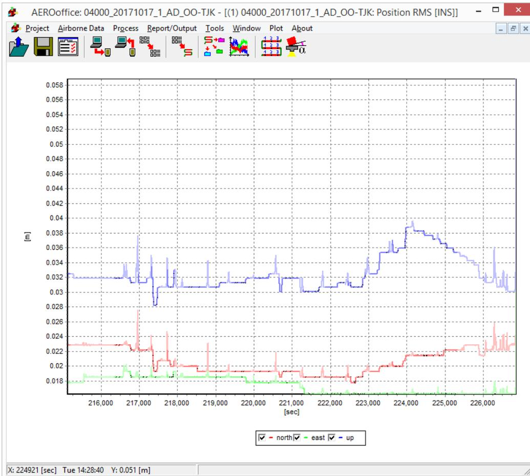
*Estimated accuracy of the trajectory after combining the GPS solution with INS.*
