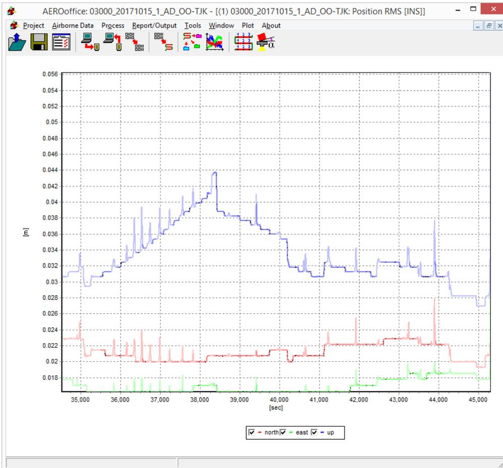
*Estimated accuracy of the trajectory after combining the GPS solution with INS.*
