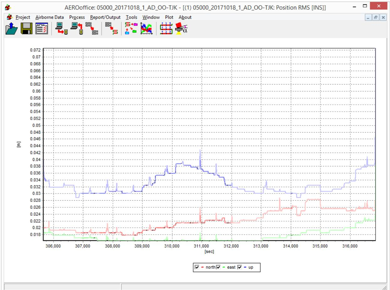
*Estimated accuracy of the trajectory after combining the GPS solution with INS.*
