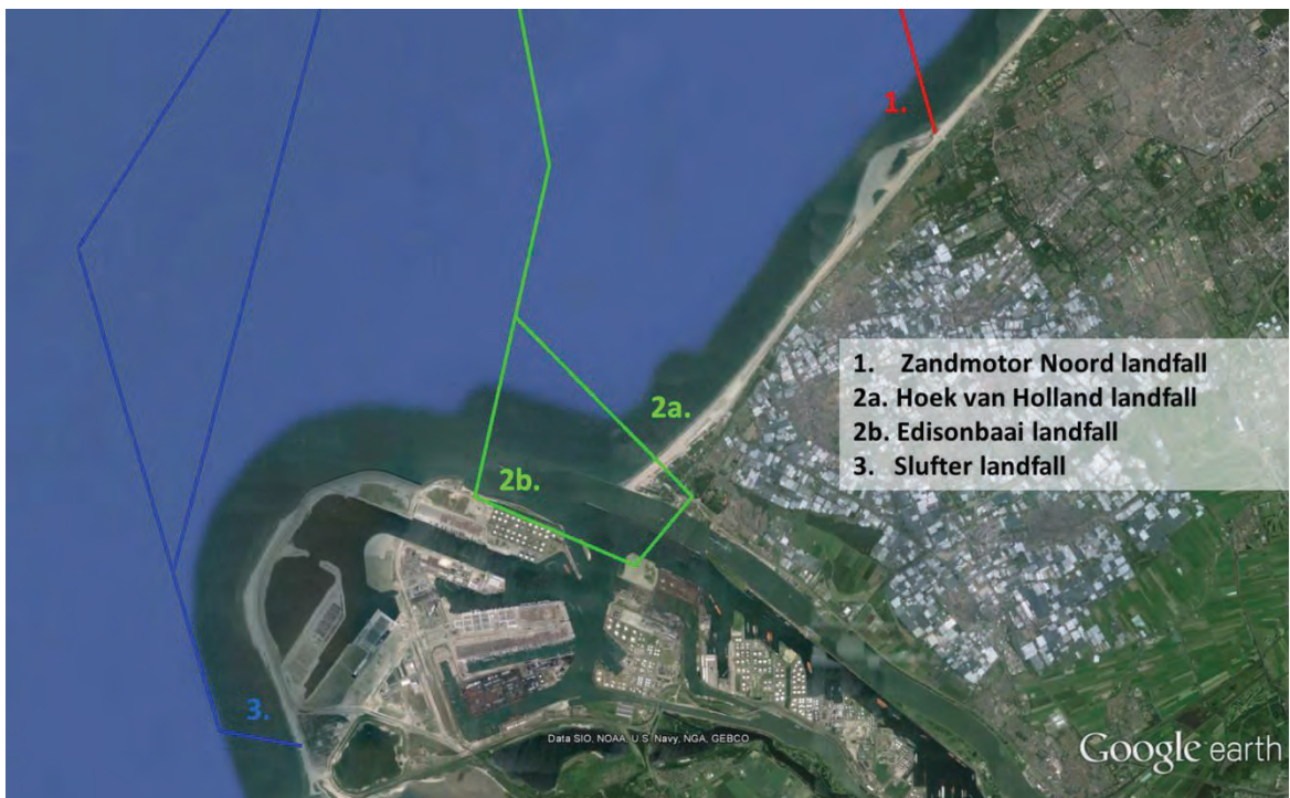
Figure 4.1 Overview of cable route landfall locations superimposed on a Google Earth image stretching from the Maasvlakte (south) to the Delfland Coast (north).
