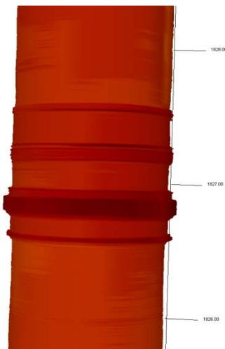
Figure 7 – 3D-calliper image of potentially undertorqued casing joint in TUB 10 at 1827 mAHbdf. The section shown is about 2.5 m long, the segment with a slight diameter increase is about 15 cm long.
