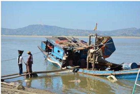
Small scale gravel extraction from main channel
