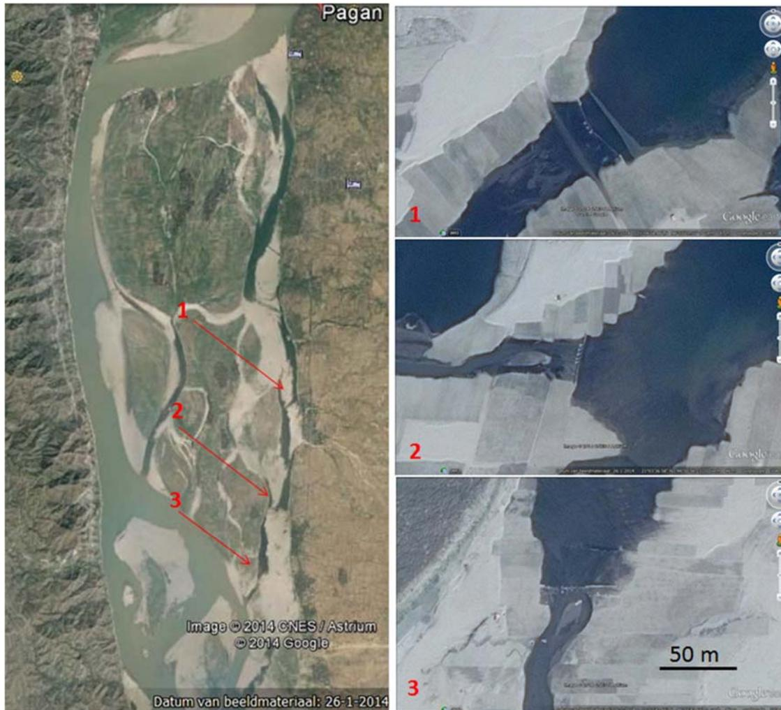
*Small weir structures that retain water in the upstream isolated water bodies of the secondary channel during low water period*
