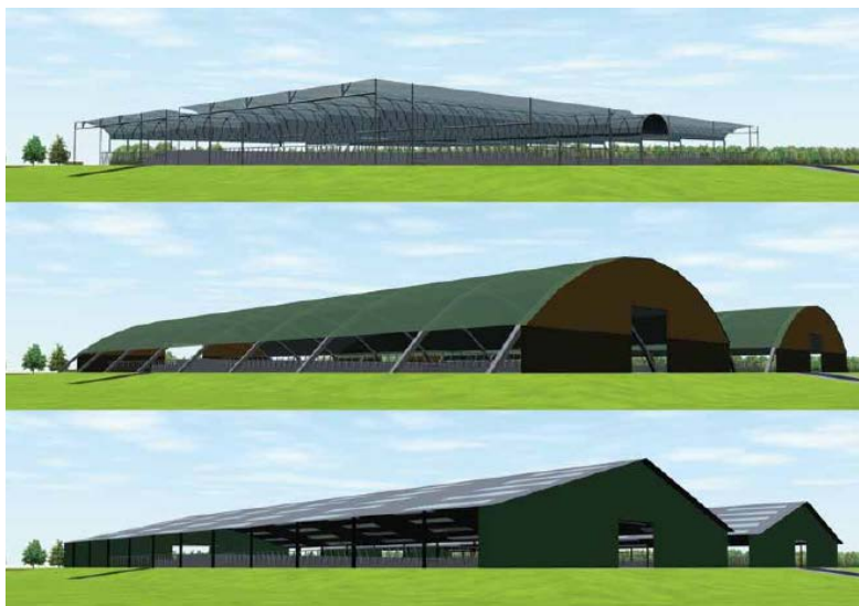
Figuur 38. Serrestallen, boogstallen en (traditionele) ligboxstallen (Bron: Courage, 2009)
