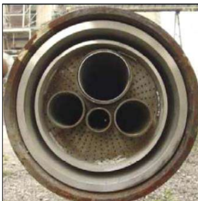
Figure 1.11: Example of a multi-channel burner [107, Belgium, 2006]
