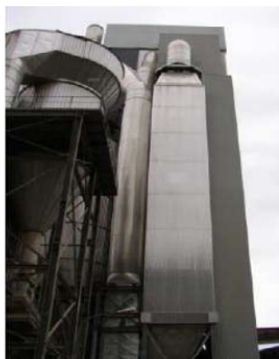
Figure 1.66: Example of an SCR installation [140, Italy, 2007]
