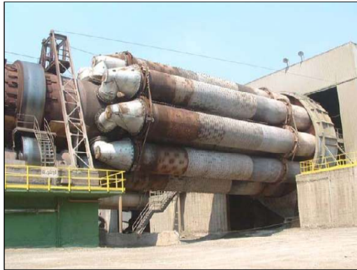
Figure 1.18: Example of a planetary cooler [45, Schorcht, 2006], [90, Hungary, 2006]
