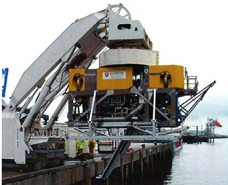
Figuur 3.11 Jet trencher (bron: Oceanteam)
