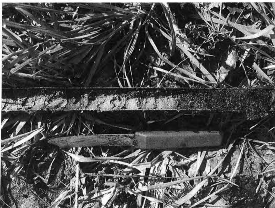
Locatie 1: Boring A2, 250-280 cm, overgang veen-zand-keileem
