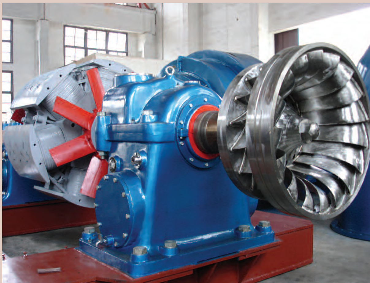
Exhibit 3.8: A Francis Turbine. (courtesy: http://hydropower.shop.co )
